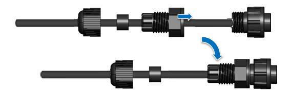
6. Insert the Seal into the Clamp Ring
