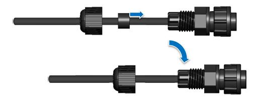
7. Push the Sealing Nut forward and Hand-tighten it to seal the assembly
