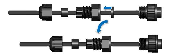
5. Wrap the Clamp Ring around the Cord Connector
