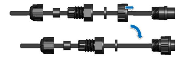
4. Insert the Gasket into the Clamping Ring
