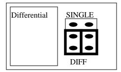
The A-823PGL/PGH offer 16 single-ended or 8 differential analog input signals. The JP3 jumper selects single-ended or differential. If JP3 jumper selects **Single-ended** position, refer to <u>Section 3.1</u> Single-ended signal of CN3 Pin Assignment (Page 40). If JP3 jumper selects **Differential** position, refer to <u>Section 3.1</u> Differential signal of CN3 Pin Assignment (Page 41).
