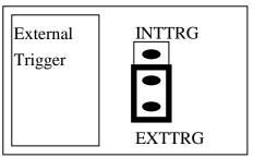
The A-823PGL/PGH supports two trigger type, **internal trigger** and **external trigger**. The external trigger comes from **ExtTrg**, **CN3 pin 17**. There are two types of internal trigger, **software trigger** and **pacer trigger**. The details information is given in the <u>Section 2.4.8</u>.
