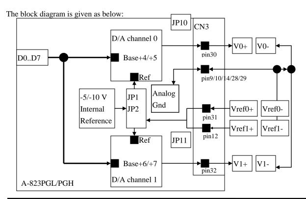
NOTE: The DA output latch registers are designed as "double buffer" structure. The user must send the low byte data first, then send the high byte data to store the DA 12 bits digital data. If the user only sends the high byte data, then the low byte data will be still the previous value. Also if the user sends high byte first then sends low byte, the low byte data of DA is still hold in the previous one.
