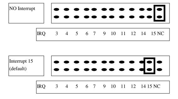
The interrupt channel <u>can not be shared.</u> The A-823 software driver can support 8 different boards in one system but only **2 of these cards** can use interrupt transfer function.
