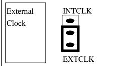
The A-823PGL/PGH has 3 independent 16 bits timer/counter. The cascaded counter1 and counter2 are used as **pacer timer**. The counter0 can be used as a user programmable timer/counter. The user programmable timer/counter can select **2 M internal clock** or **external clock ExtCLK**, **CN3 pin 37**. The block diagram is given in the <u>Section 2.6</u>. The clock source must be very **stable**. It is recommended to use internal 2 M clock.
