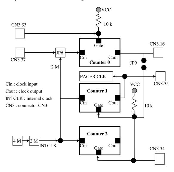
The counter0, counter1 and counter2 are all 16 bits counter. The COUT of counter 0 can control counter 1 gate by JP9 setting. The counter1 is a 16 bits timer is used as <u>pacer timer</u>. The software driver, A823\_Delay(), uses counter 0 to implement a machine independent timer for settling time delay (<u>Section 2.4.6</u> and <u>Section 2.4.7</u>). If user doesn't use A823\_Delay(), the counter0 can be used as a general purpose timer/counter.
