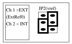
If JP2 jumper is configured in **INT** position, the JP1 jumper must be configured to provide -5 V or -10 V internal reference voltage for D/A (see Section 2.3.1).
