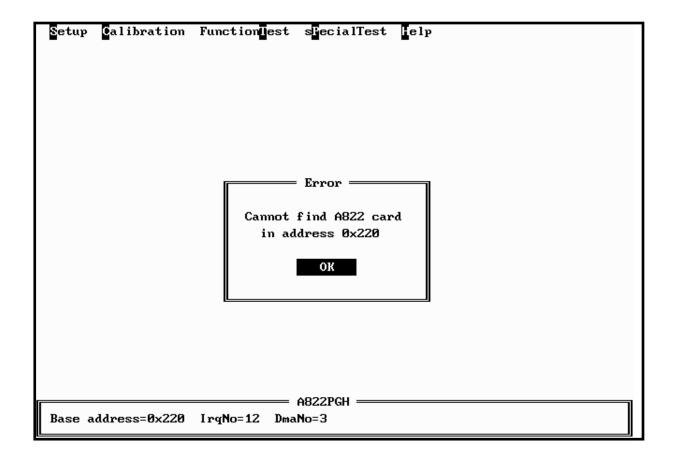
Although you can continue the A-823DIAG by press any key, it is recommended to correct this situation by setting the proper jumper setting. Because many operation in the A-823DIAG, the I/O base address is check firstly. And it don't work if the error occurs
