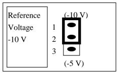
Select (-5 V) : Voltage output range =  $0 \sim +5$  V<sub>DC</sub> for both D/A channels Select (-10 V) : Voltage output range =  $0 \sim +10$  V<sub>DC</sub> for both D/A channels Note that JP1 is validate only if JP2 select D/A internal reference voltage
