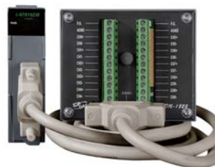
I-87019ZW-G/S2 = I-87019ZW Connect DN-1822 Directly and CA-252518D-1 1.8 m Cable
