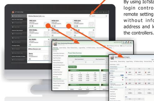
By using IoTstar, you can directly login controller to perform remote setting and maintenance without information of IP address and login password of the controllers.
