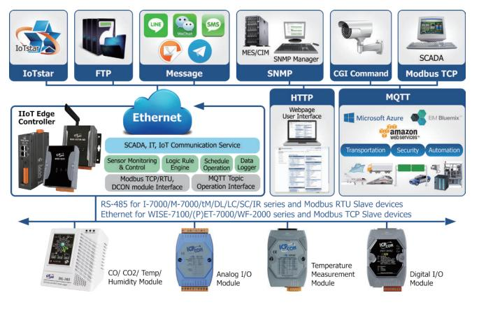
Based on the built-in Edge Computing Engine WISE provide, users can access Web server on WISE through browser to perform the tasks such as logic rule edition, download and execution to meet the requirement of real-time Edge Computing operation at the field site.
