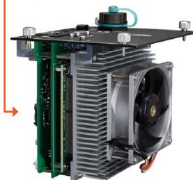
The temperature of the entire CPU can be reduced by another 10°C with larger heat sinks and fans, extending the service life of electronic components. The fan has been specially selected for the long-life type, with a lifespan of 180,000 hours (about 20 years).
