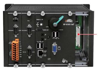
I/O Slot (COM1) **I-9K/I-97K Bus** For I-9K/I-97K Module
