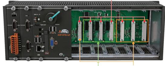
e-Bus or I-9K/I-97K Bus For e-9K Module or I-9K/I-97K Module
