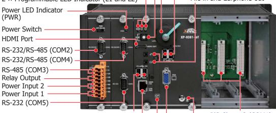
USB Port  $\times$  2 (P1 and P2) Ethernet (LAN2) VGA Port
