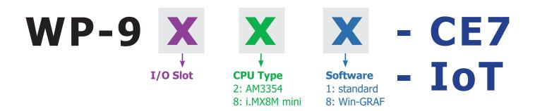
The WP-9000-CE7 series has a built-in Windows CE 7.0 operating system and supports a variety of software development tools: VB.Net 2005/2008, Visual C#.NET 2005/2008, Win-GRAF. In addition to the small operating core of Windows CE 7.0, it provides a Hard Real-Time, and deeper interrupt processing capabilities that is very suitable for stable and critical control.
