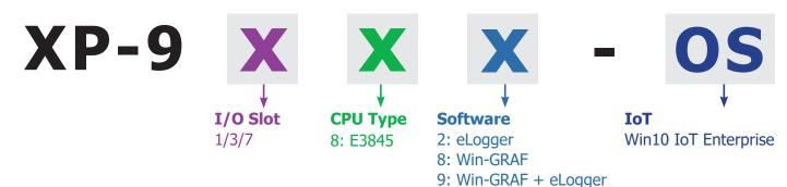
XP-9000-IoT has a built-in Windows 10 IoT Enterprise operating system, which can support both the Universal
