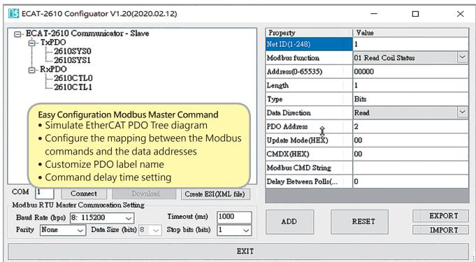
▲ ECAT-2611 provides a Modbus RTU command deployment tool that can be configured in 5 minutes.
