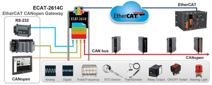
▲ Anything can be connected to the EtherCAT master via ECAT-2614C as long as it is a CANopen device
