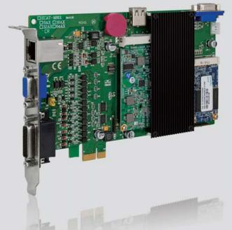
▲ ECAT-M801 handles motion control, allowing the PC system to focus on other tasks
