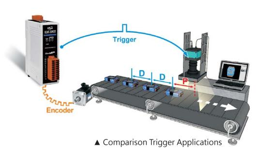
The location comparison function can be accessed via software or through a dedicated DI. By connecting its DO to the DI of the ECAT-2072IT, an external PLC or controller can enable/ disable the comparison function of the ECAT-2072IT. The image on the left depicts a simple location comparison application with a comparison function that can be enabled/ disabled via software or hardware.
