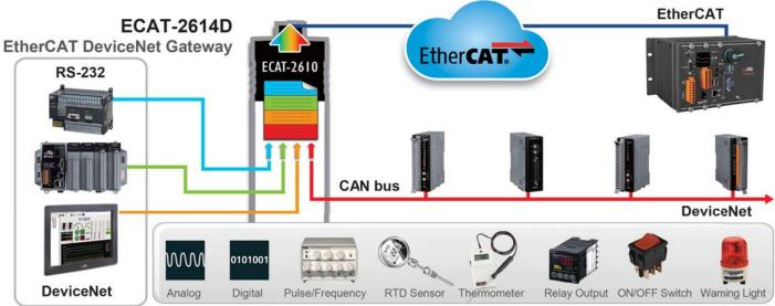
▲ Anything can be connected to the EtherCAT master via ECAT-2614D as long as it is a DeviceNet device
