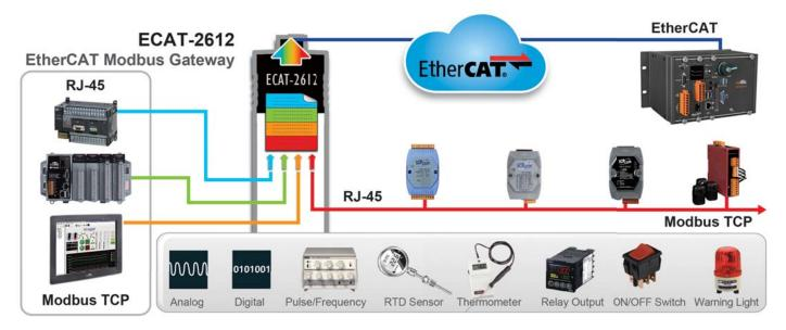
▲ Anything can be connected to the EtherCAT master via ECAT-2612 as long as it is a Modbus TCP device
