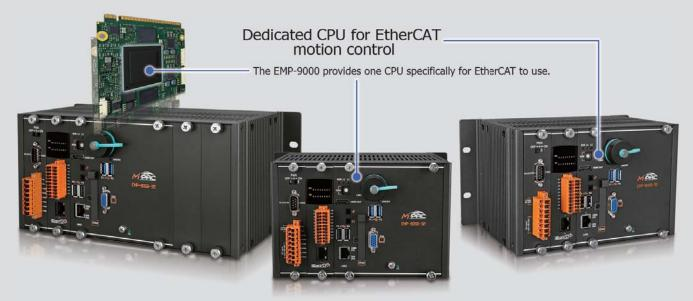
▲ The EMP-9000 series EtherCAT motion controller with an all-metal case meets users' most stringent requirements for anti-interference capability and system size.
