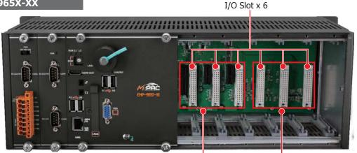
e-Bus(x4,x1) or I-9K/I-97K Bus (apply to e-9K module or I-9K/I-97K module)
