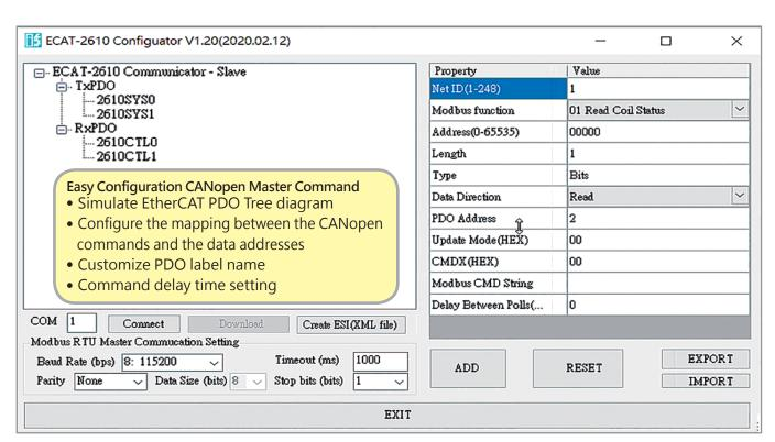
▲ ECAT-2615C provides a CANopen command deployment tool that can be configured in 5 minutes.
