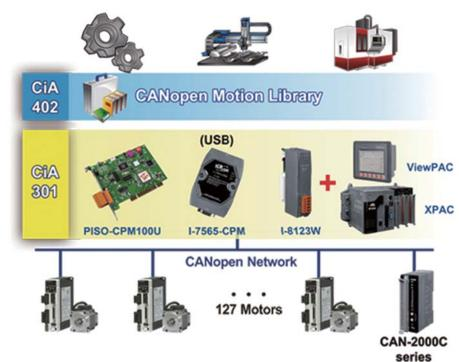
A large number of CANopen-based motors can be linked together so that multi-axis motion control via a single host becomes achievable. While controlling the motors, CANopen-based remote I/O modules that comply with the CiA 402 standard can also be accessed at the same time. Therefore, developing a motion control application becomes easier and more convenient.
