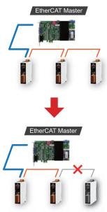
▲ If there is no diverter, the module will stop working when the cable disconnects.
