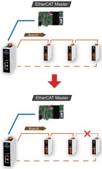
▲ When a diverter is available, the module can return to normal operation through cable redundancy.
