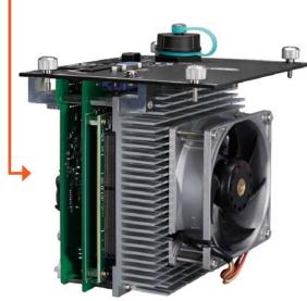
The temperature of the entire CPU can be reduced by another 10°C with larger heat sinks and fans, extending the service life of electronic components. The fan has been specially selected for the long-life type, with a lifespan of 180,000 hours (about 20 years).
