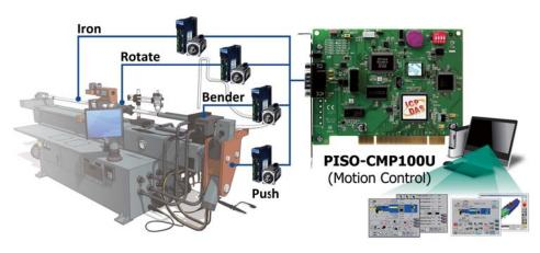
In the machine, there are sixaxis motors which use distributed CANopen motion control. During the tube bending process, the two axes of the feeding and radial bending are designed to be interpolation motion. The cycled processes are designed to prevent the metal tube broken and rebound. It greatly improves the yield of bending. The CANopen motion also help to shorten the development time at the design stage.
