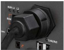
▲ Secured RJ45 Connector Kit
