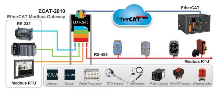
▲ Anything can be connected to the EtherCAT master via ECAT-2610 as long as it is a Modbus RTU device
