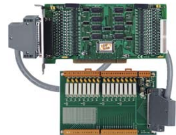
PISO-P32C32 with DB-16P16R: 16-ch input terminal and 16-ch Relay (3A, Form A) board, 1 m 電纜 .
