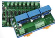
Current Sensor Voltage Attenuator
