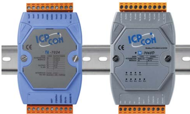
導軌安裝 (DIN-Rail Mounting)
