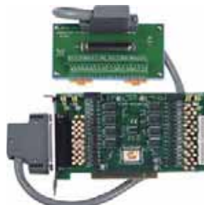
PISO-P64 with DN-37: D-sub 37-pin daughter board with 1 m 电缆.
