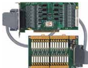
PISO-C64 with DB-32R: 32-ch relay (3A, Form A) board, 1m 电缆.
