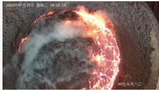
Water-bearing steel slag poured into slag tanks and generated air explosion
