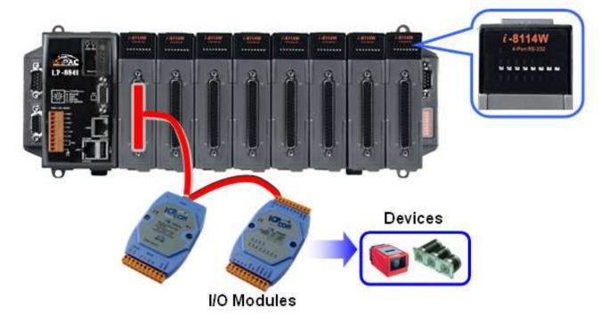
To get more RS-232/485/422 ports, user can plug one or more "multi serial port module" in the I/O slot.
