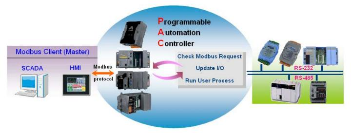
The LinPAC controller also provides a Modbus SDK based on the C language, which can be used to integrate several serial devices. Thus, the controller can be used as either a Modbus/TCP slave or a Modbus/RTU master. The Modbus SDK can not only be used to communicate with Modbus/RTU devices but can also use the easy-to-use register-based programming method.
