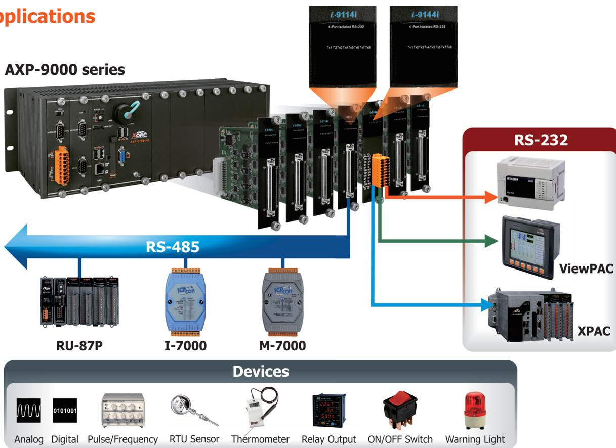
To get more RS-232/485/422 ports, user can plug one or more "multi serial port module" in the I/O slot.
