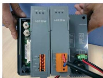
CANBUS Communication module I-8120W
