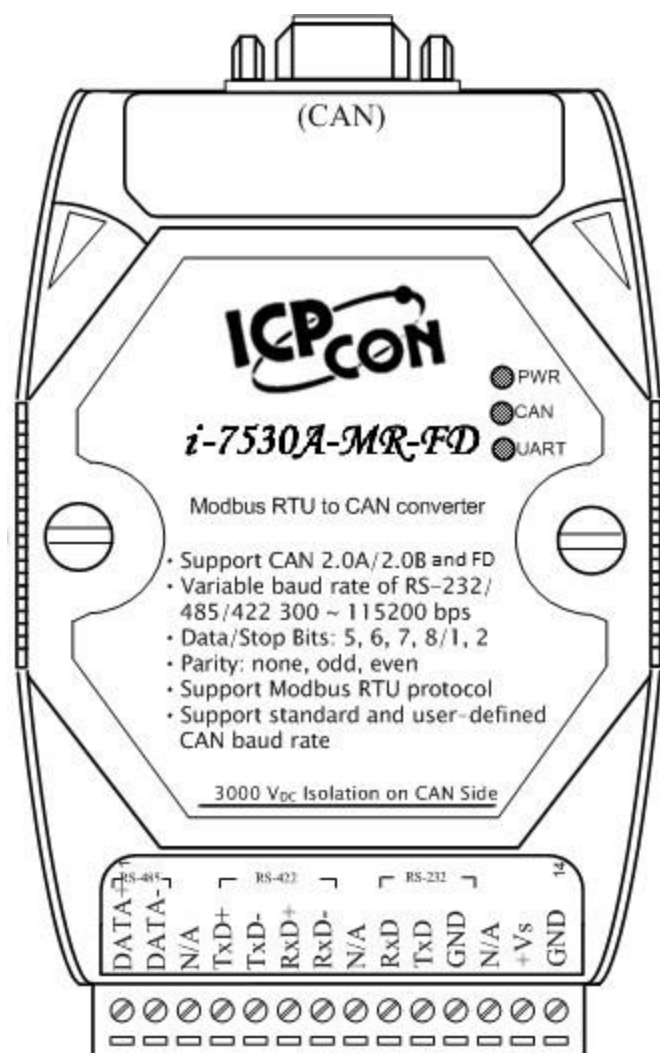
Figure 2-1: Hardware profile of the I-7530A-MR-FD
