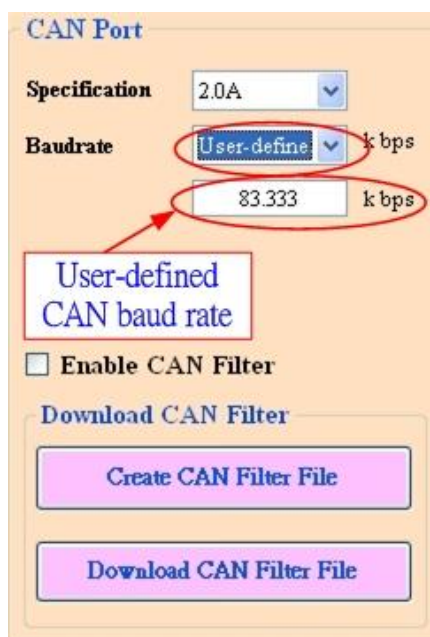
Figure 6-1: User-defined CAN Baud Rate for I-7530A-MR-FD
