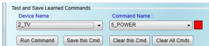
▲ Figure 3-16 Test & save IR commands section.
