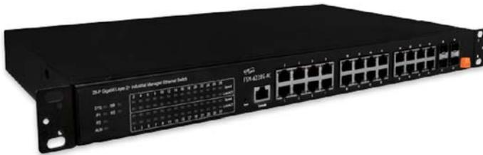
FSM-6228G is a L2 Managed Switch that meets all IEEE 802.3ab/u/x/z Gigabit, Gigabit Ethernet and Ethernet specifications. It provides 24 gigabit Ethernet ports (10/100/1000 Mbps TP) 4 SFP ports.
