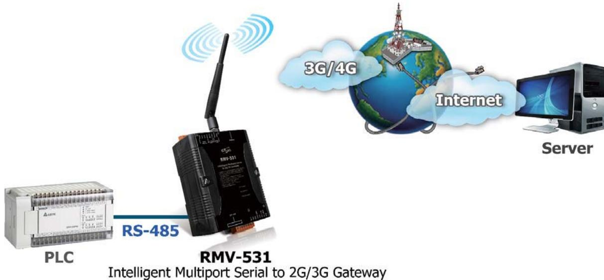
It is a SMS and voice alarm system in machine application. The Machine can report or inform the worker to fix the machine when it break down.
