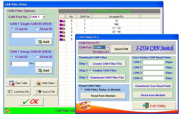
This utility configures the CAN filter and user-defined CAN baud rate. It can save the CAN filter configuration as file and would be import to another I-2534.
