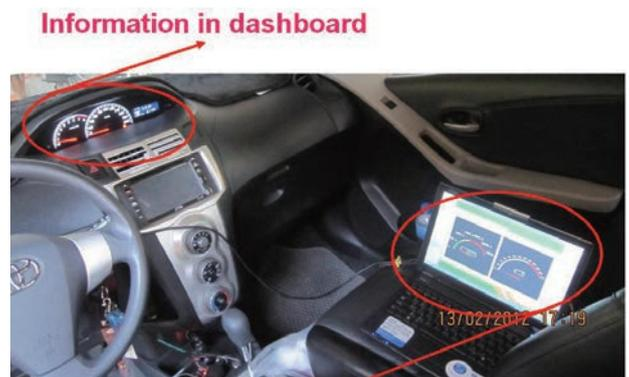
Monitor the CAN data of the engine and vehicle Speed via the I-7565-H2.
