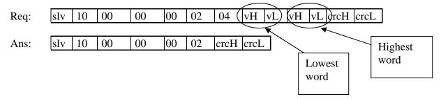
To read / write float (4 bytes) is very similar to read / write long word. The difference is the variable should be declared as "Real" type, and the next network address No. should not be assigned to any other variable.
