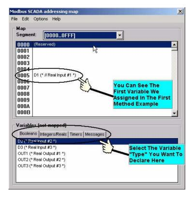
To assign the other variable address click on an unassigned "Map Segment" number, and then double click on the variable you want to assign to the address and the variable will automatically assign itself to the "Map Segment".
