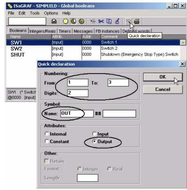
Link Variables to the associated channels of connected I/O modules.
