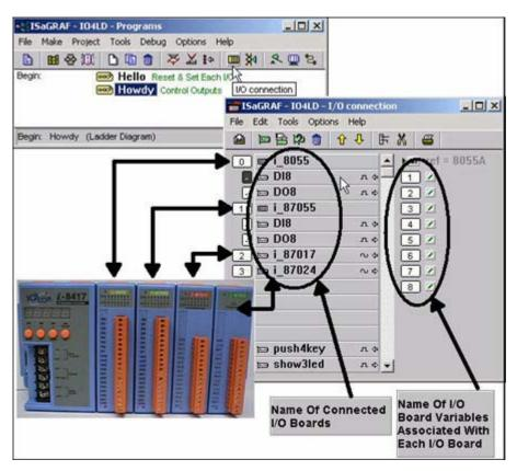
Declare Variables associated with the channels of connected I/O modules. You may refer to section 2.1.1.3 Example:
