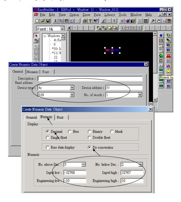
Click on "Numerical Input", set "Device Type" to "4x", "Device address" to 10, "BIN", "Number of words" to 1, "**Trigger Device Type" to "LB", "Trigger Device address" to "9000",** "No. above Dec" to 7, "No. below Decimal" to 0, "Input low" to –32768, "Input high" to +32767. And then select the prefered shape.
