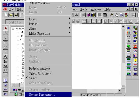
PLC type should be set to "MODBUS RTU", Serial port set to "RS232", Data bits set to "8 Bits", Stop bits set to "1 Bit", Baud rate set to "19200", Parity set to "None", PLC station No. set to be equal to the Net-ID of the I-8xx7 (set to 1 in this example).
