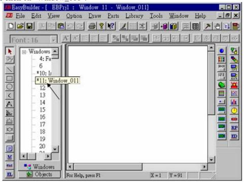
Create a change-window "Function Key" as former method to change to "Window No." = 10, and Labeled as "BACK".
