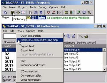
When you click on "Modbus SCADA Addressing Map" (SCADA is an industrial process control acronym that stands for "Supervisory Control And Data Acquisition") the "Modbus SCADA Addressing Map" window will open.
