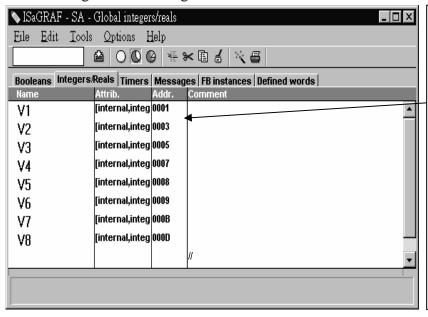
V1 is assigned to a network address "1". If the network address "2" is not assigned to any other variable, V1 will occupy a long word (4 bytes) in the Modbus transportation formate.
