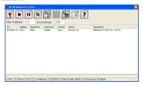
10. Click the name of the module to open the Configuration dialog box and configure the module.
