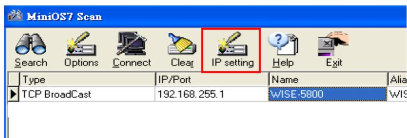
Figure 2-3 : IP Setting button on MiniOS7 Scan
