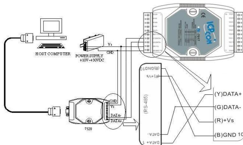
Figure 2-5 : I-7000 module connection via RS-485 line
