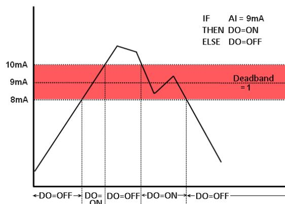
**Figure 4-12 : AI Deadband Operation(= a numerical value)**
