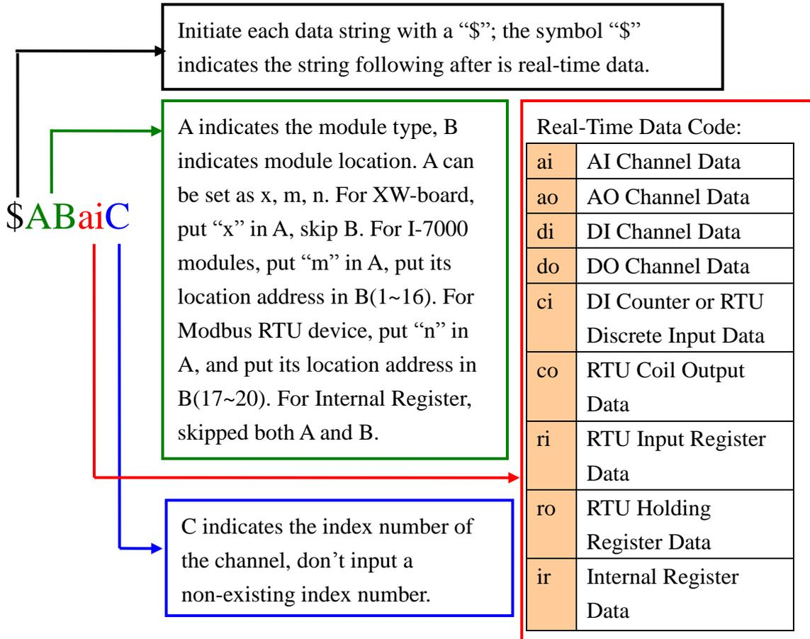
Figure 5-16 : SMS Command Data Retrieve Coding Rules
