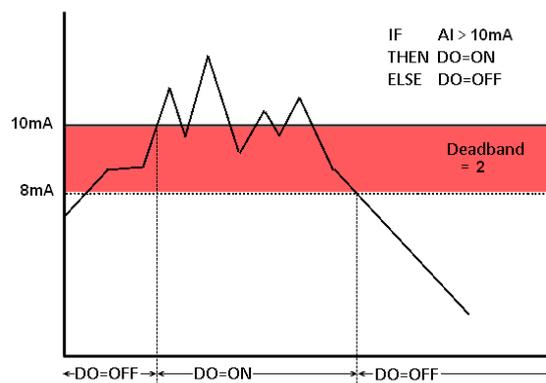
**Figure 4-10 : AI Deadband Operation(> or >= a numerical value)**
