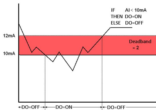
**Figure 4-11 : AI Deadband Operation(< or <= a numerical value)**
