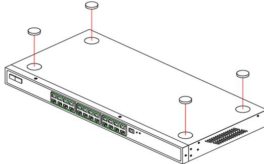
**Step2.** Set the device on a flat surface near an AC power source, making sure there are at least two inches of space on all sides for proper air flow.
