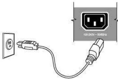
**Step1.** Insert the power cable plug directly into the AC Socket located at the back of the switch.
