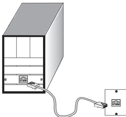
**Step2.** If the device is a network card and the switch is in the wiring closet, attach the other end of the cable segment to a modular wall outlet that is connected to the wiring closet. (See the section “Network Wiring Connections.”) Otherwise, attach the other end to an available port on the switch.
