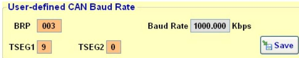
The screenshot shows a configuration window titled "User-defined CAN Baud Rate". It contains four input fields: "BRP" with the value "003", "TSEG1" with the value "9", "TSEG2" with the value "0", and "Baud Rate" with the value "1000.000 Kbps". A "Save" button is located at the bottom right of the window.
