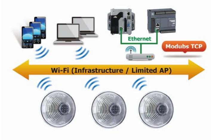
Figure 1-1: Application architecture for the ALM-Horn-WF(-BR)
