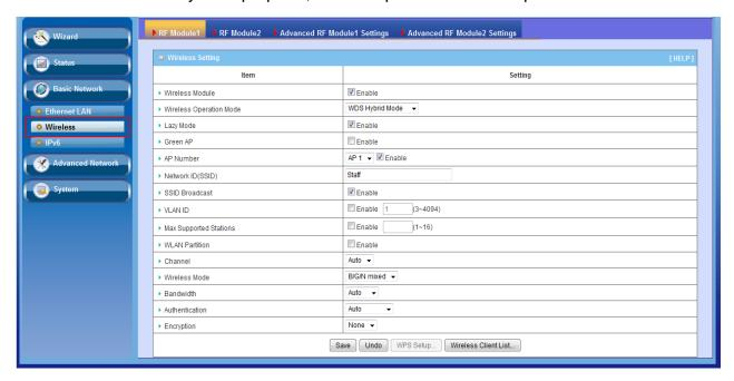
The embedded RF Module1 is a IEEE 802.11b/g/n compliant 2.4GHz Wireless Module and RF Module2 is a IEEE 11g/n/ac compliant 5GHz Wireless Module.
