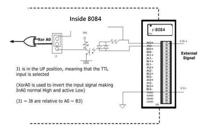
Isolated or TTL input is selected by using JP1 to JP3 as indicated below:
