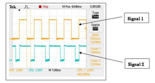
Input signal=500Hz & Low Pass Filter Enabled=1µs
