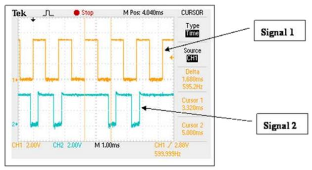
Input signal=600Hz & Low Pass Filter Enabled=1µs
