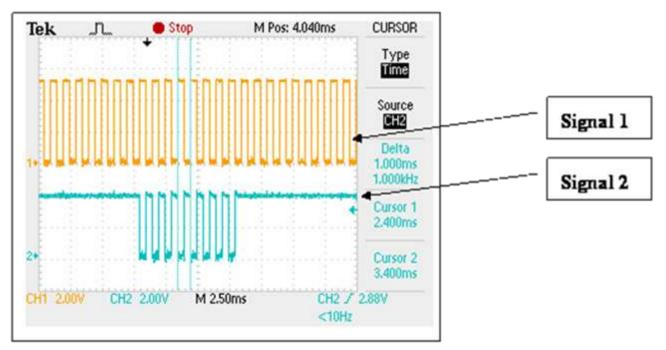
Input signal=1000Hz & Low Pass Filter Enabled=1µs
