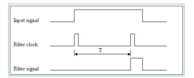
Note: the filter signal is shorter than the original input signal.
