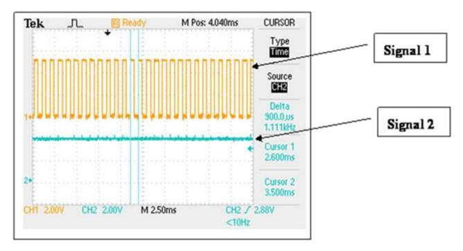
Input signal=1100Hz & Low Pass Filter Enabled=1µs
