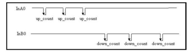
When InA0 is used as a UP\_clock and InB0 is used as a DOWN\_clock. The counter\_0 will be increased by one for every falling edge of InA0 and decreased by one for every falling edge of InB0.
