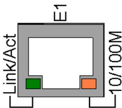
The MDC-700 is equipped with a RJ45 port for Ethernet LAN connection. When 100BASE-TX is operating, the 10/100M LED is lit orange. When 10BASE-T is operating or the machine is not connected to the network, it is turned off. When an Ethernet link is detected and an Ethernet packet is received, the Link/Act LED is lit green.
