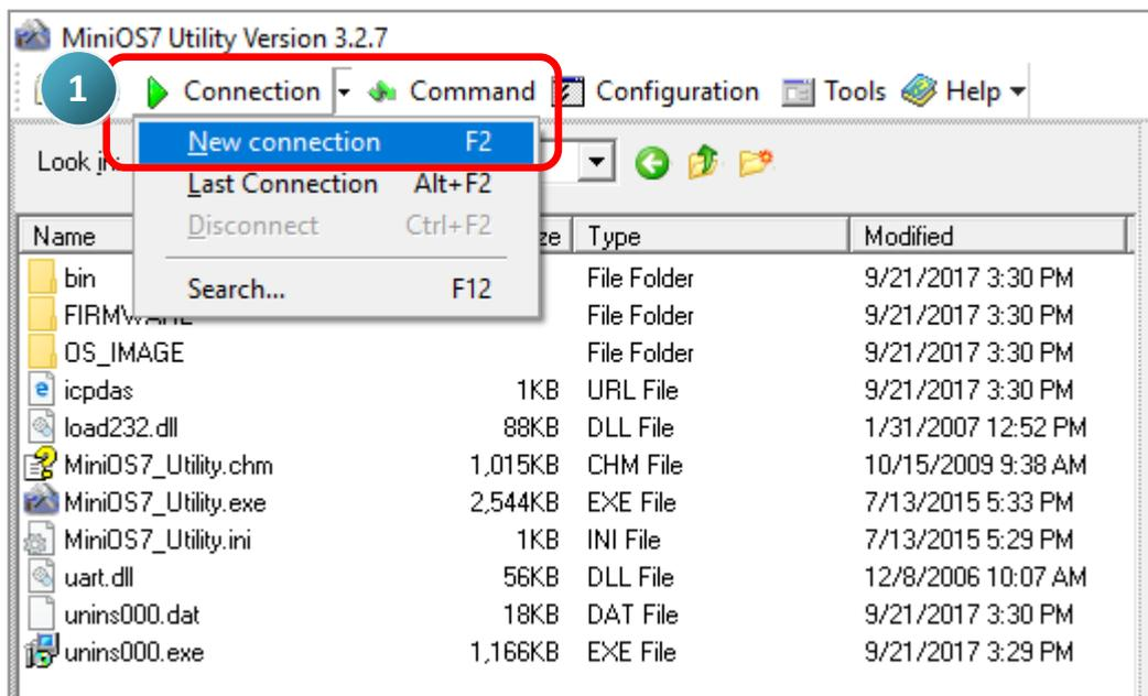
On the **“Connection”** tab of the **“Connection”** dialog, select **“TCP”** from the dropdown list, type the IP address of MDC-700, and then click OK button.
