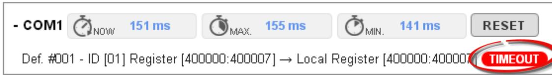
◆ **Situation #1:** The slave device is not active or the transfer function of the slave site may fail.
