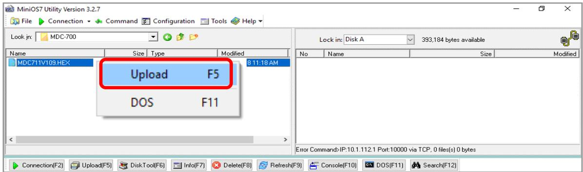
Step 6: Wait until the firmware update is finished, and then power cycle the MDC-700.
