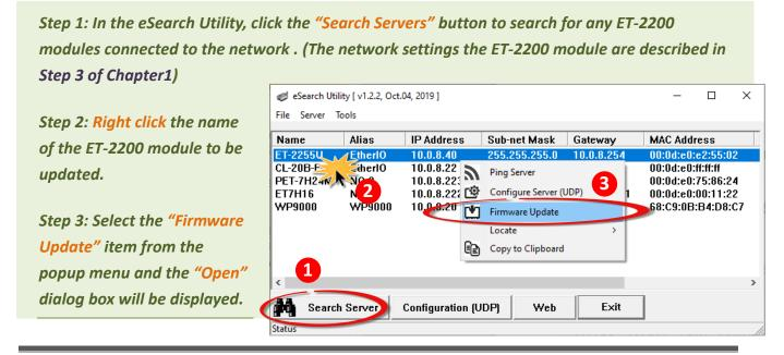
Step 4: In the "Open" dialog box, select the firmware file (ET2200.dat) that will be used to update the module and then click the "Open" button.
