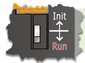
Step 11: Once the update is complete (i.e., when the progess indicator reaches 100%), set the "Init Switch" to the "Run" position.
