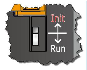
Step 2: Set the "Init Switch" to the "Init Mode" position.
