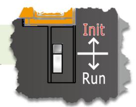
Step 9: Power-on reset the ET-2200 module in "Init Mode" to initiate the update.
