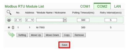
Please note: if fail to scan the I/O modules, please make sure the RS-485 cable is properly connected. And then go to Step 1: "System Setting" $\rightarrow$ "I/O Interface Setting" to make sure the settings of the COM Port that are connected to the I/O Module are accurate. After all settings are completed, click "Save" button to save the changes and repeat Step 3.a to perform scanning of the I/O modules again.
