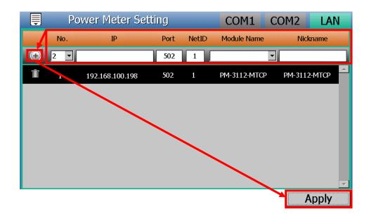
(8) After complete the setting of Modbus RTU/TCP power meter, please click the "Save the Settings" on the "Module Setting" menu, and then the new setting will take effect.
