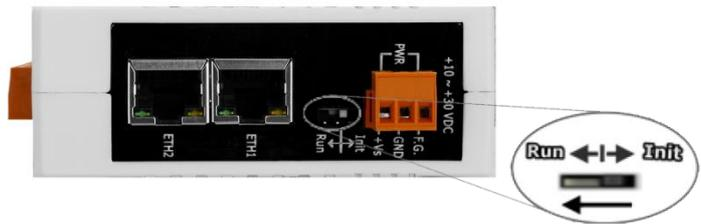
3. Connect both the DS-2200 and the Host computer to the same sub-network or the same Ethernet Switch, and then supply power (PoE or +12 to +48 VDC) to the DS-2200.
