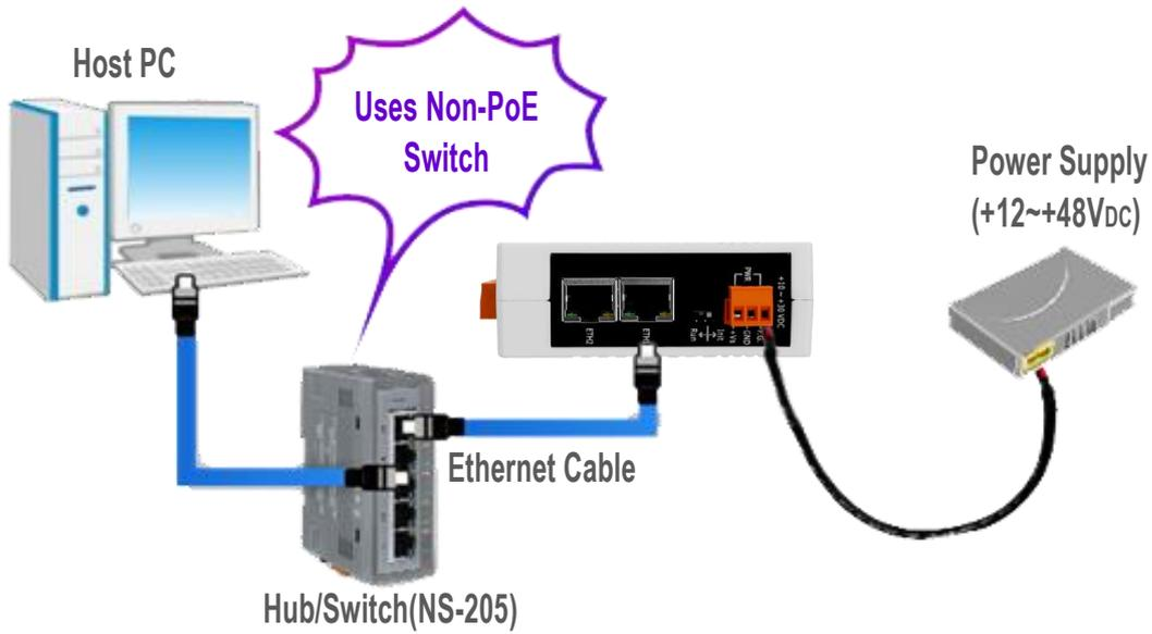
4. Verify that the **System LED** indicator is flashing.
