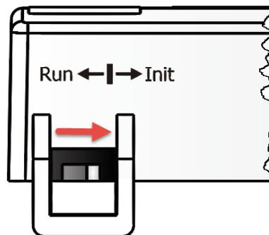
For tDS-700/DS-2200 series modules, the operating mode switch is set to the **Run** position by default. In order to update the firmware for the tDS-700/DS-2200 series module, the switch must be moved from the **Run** position to the **Init** position. The switch must be returned to the **Run** position after the update is complete.
