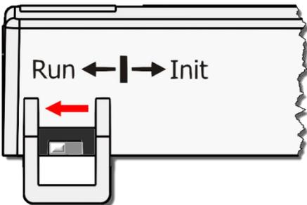
**Step 4** Reset the Init/Run switch on the tDS-700/DS-2200 module to the "Run" position and reboot the device.
