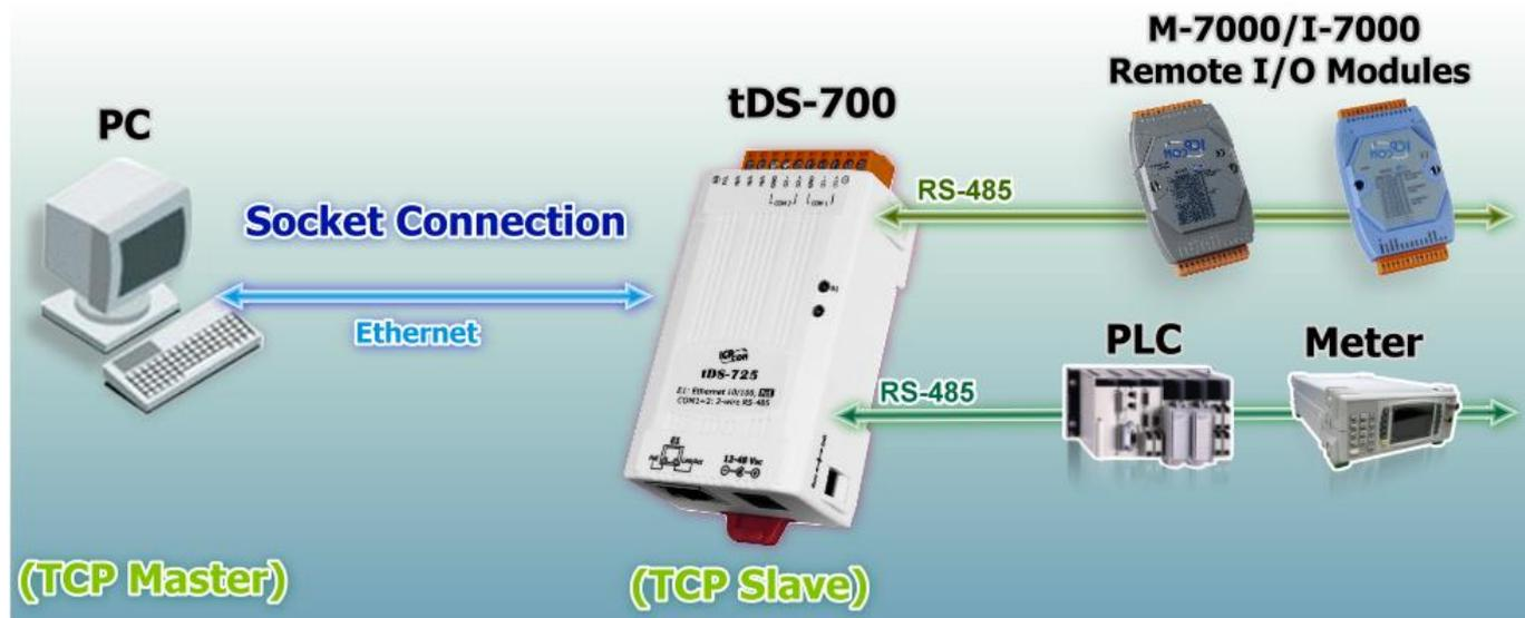
tDS-700/DS-2200 series module can accept the TCP connection (include raw data) directly, it also can communicate with TCP client and Serial Device in this way.
