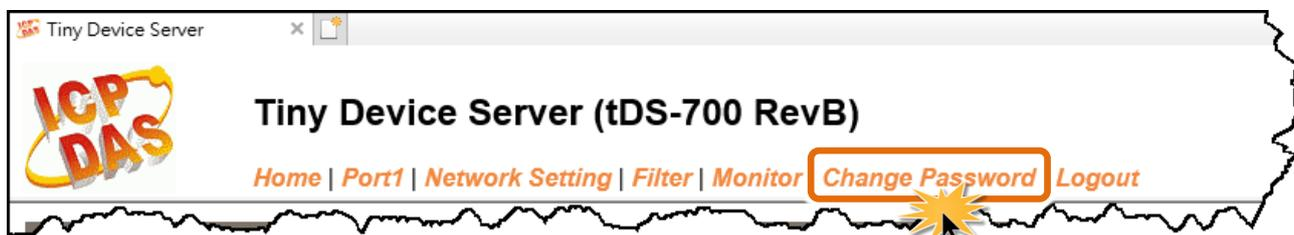
After clicking the **Password** tab, the **Change Password** page will be displayed. To change a password, first enter the old password in the “**Current password**” field (use the default password “**admin**”) and then enter a new password in the “**New password**” field. Re-enter the new password in the “**Confirm new password**” field, and then click the “**Submit**” button to update the password.
