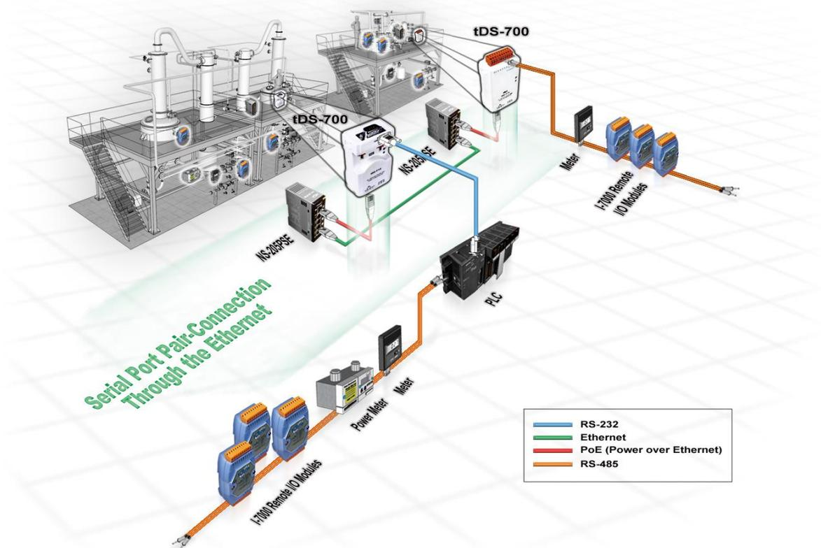
In harsh industrial environments, the tDS-700/DS-2200 series (for i version) also adds 3000 V<sub>DC</sub> and +/- 4 kV ESD protection component that diverts the potentially damaging charge away from sensitive circuit to protects the module and equipment from the sudden and momentary electric current.
