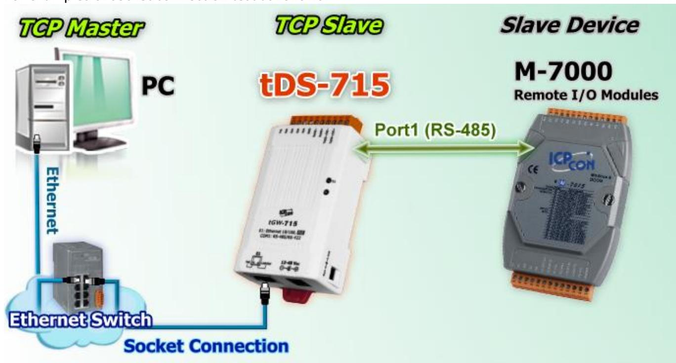
1. Confirm that the tDS-700/DS-2200 modules are functioning correctly. Refer to [Chapter 3 “Getting Started for tDS-700 series”](#), [Chapter 4 “Getting Started for DS-2200 series”](#) for more details.
