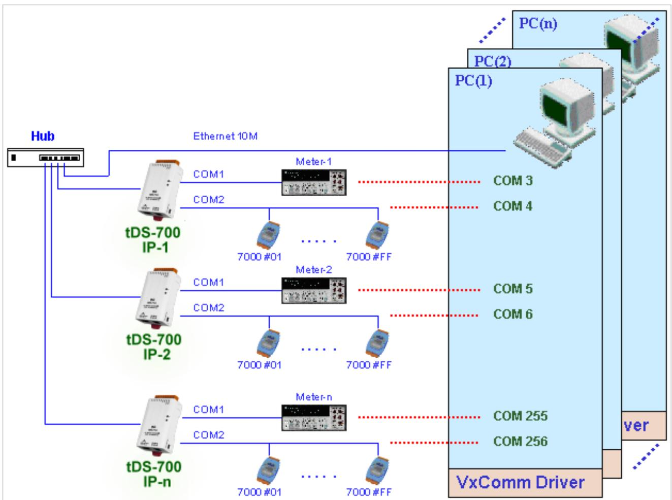
The VxComm driver controls all the details of the Ethernet TCP/IP programming technique, meaning that, with the assistance of tDS-700/DS-2200 and VxComm technology, your COM Port program will be able to access your serial devices through the Ethernet in the same way as through a COM Port.
