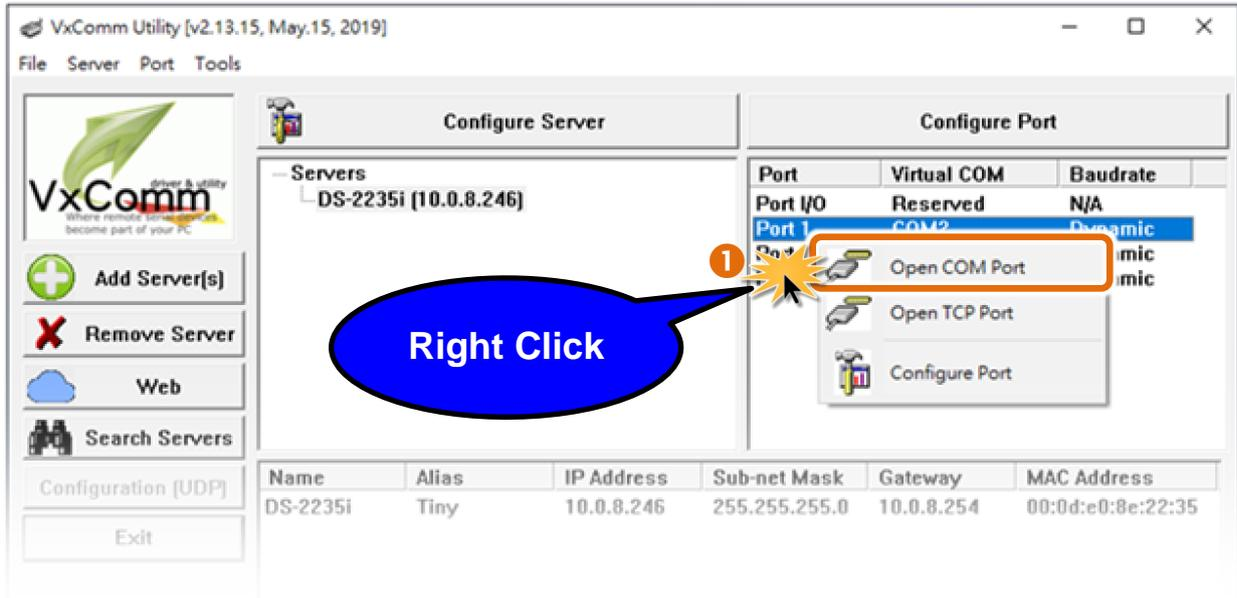
2. Check that the configuration of the COM Port is correct and then click the **“Open COM”** button.
