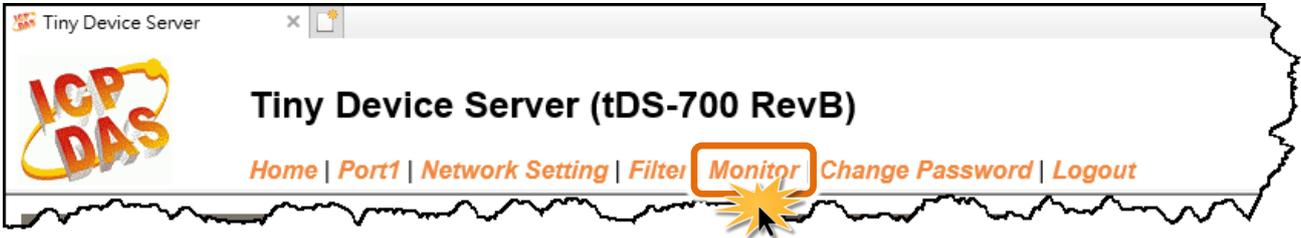
After clicking the **Monitor** tab, the Current Connection Status page will be displayed showing detailed information regarding the current status of the serial port connection settings for the tDS-700/DS-2200 module.
