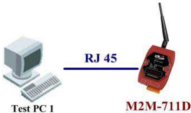
Ethernet default value is 192.168.1.217. The PC and M2M-711D have to set setting in the same network segment. The example of connection setting will be described below and Microsoft Windows XP Professional SP2 is used.
