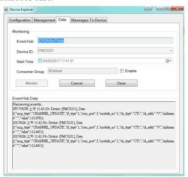
xi. Go to the "Main Page >> Power Meter Information >> I/O(Tab)" page to observe that the relay status changes when PMC-5231 gets the message send by Device Explorer.
