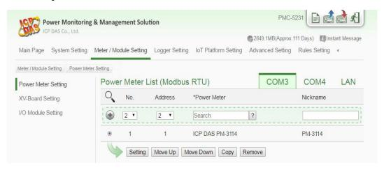
iv. Complete the settings, download the setting to PMC-5231, and then go to the "Main Page" to check the communication status with the power meter.
