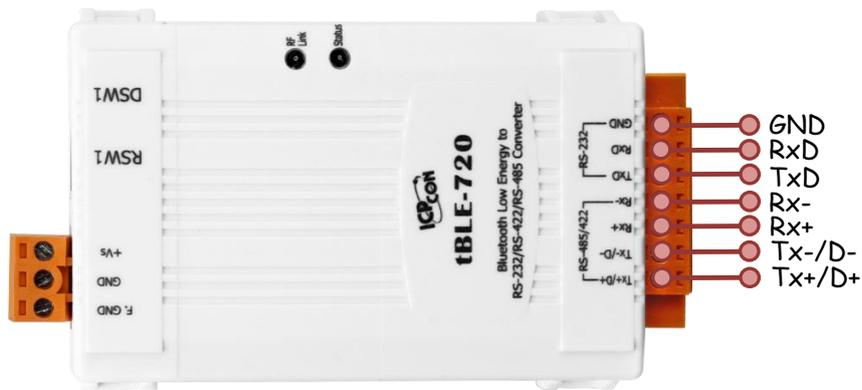
Figure 2-5. Communication connector
