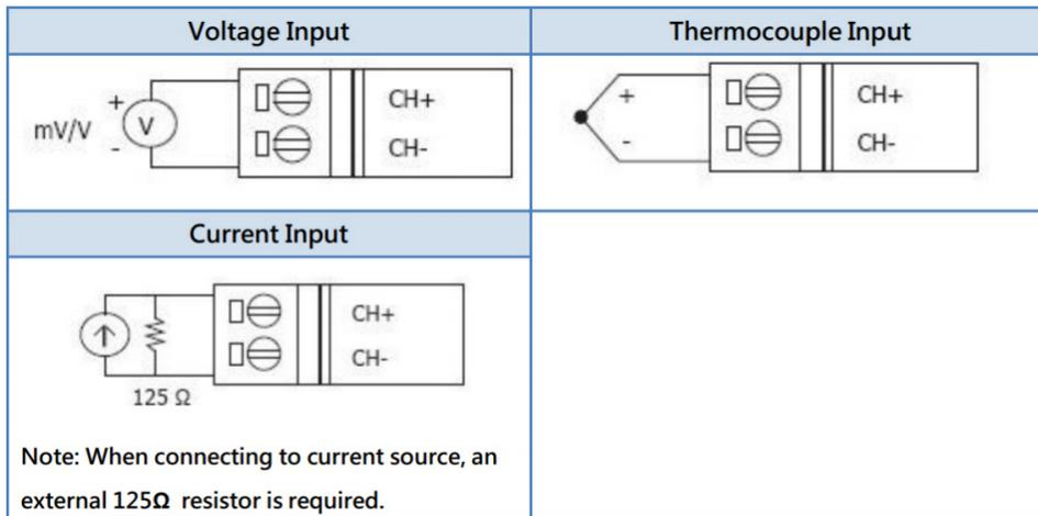
Figure 5: Wire connections
