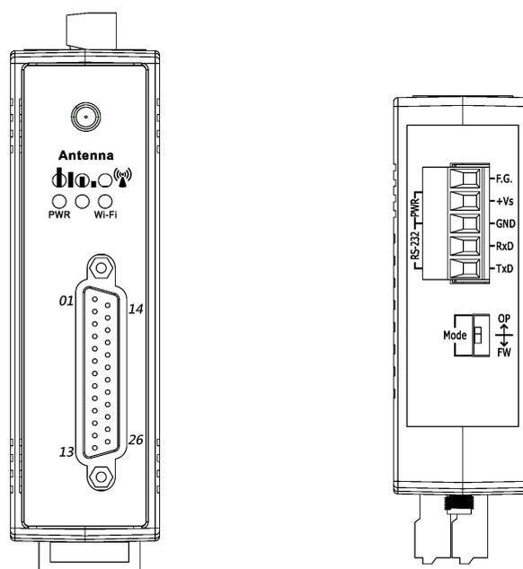
Figure 1: Appearance of the WF-2019
