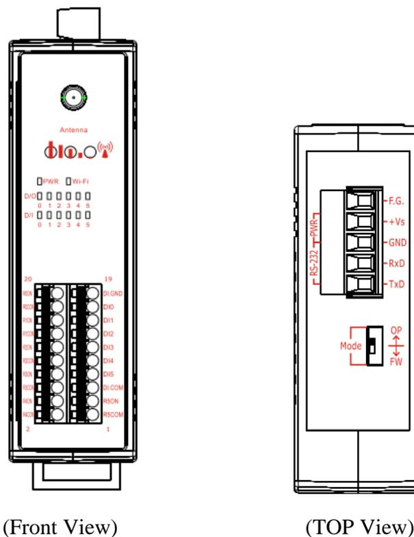
Figure 1: Appearance of the WF-2060
