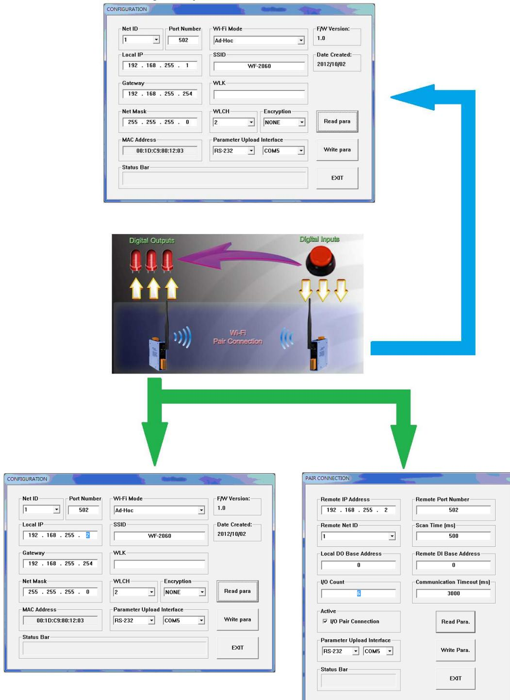
Figure 20: Pair connection architecture and setting interface
