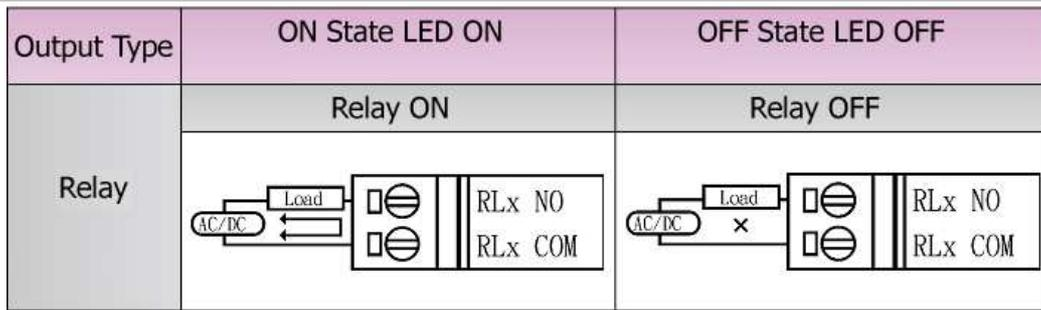
Figure 5: DO wire connection
