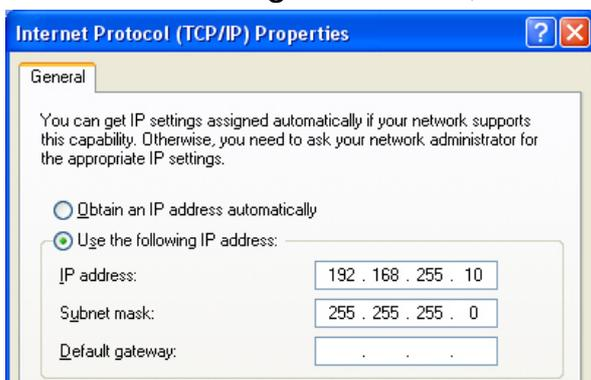
Figure 5: IP configuration interface
