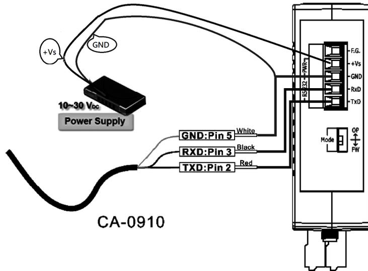
Figure 2: Power and Serial port wire connection
