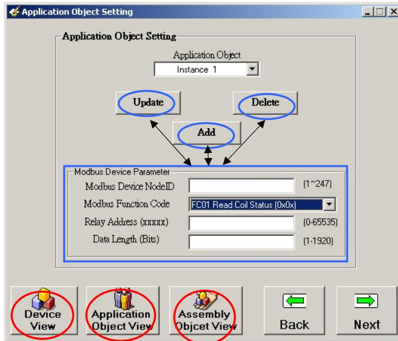
**Step 7:** After the configuration of Modbus devices parameters, press the “Next” button and start to build the specific EDS file for the I-7242D. Set the EDS file information and give it a description in the description box. Then set the poll, strobe-bit and COS/Cyclic I/O connection path for the I-7242D.
