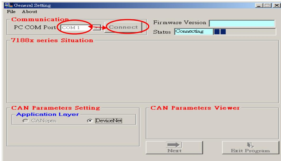
**Step 5:** After reading parameters from EEPROM, a related information dialog box will be displayed. Then you can set the CAN and COM port parameters to what you need.
