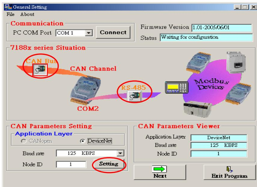
**Step 6:** After setting the CAN and COM port parameter, press the “Next” button to start to set their Modbus devices parameters. Users can use the add button, erase button, update button or delete button to modify their Modbus devices parameters. And users can view the information of devices, application object and assembly object by clicking these “View” buttons.
