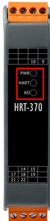
Figure 2.5: LEDs on HRT-370
