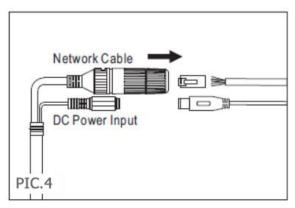
• Connect the RJ-45 Ethernet cable with a waterproof connector
