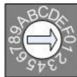
Figure 2-3 Baud rate rotary switch
