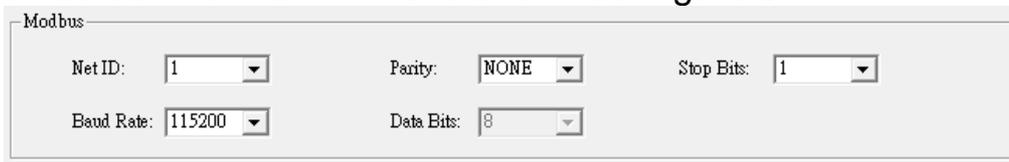
Figure 6: Modbus configuration screen
