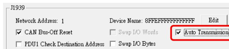
Figure 11: J1939 Auto Transmission function screen
