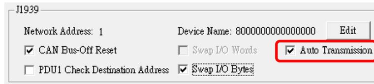
Figure 12: J1939 Auto Transmission function screen
