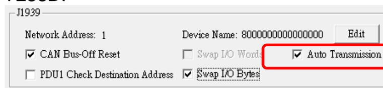
Figure 13: J1939 Auto Transmission function screen
