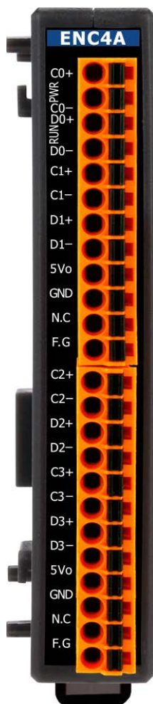
Figure 4: EC4-ENC4A side view with encoder inputs
