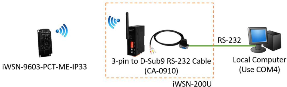
**Figure 4-8: The system architecture of the iWSN Utility Demo**
