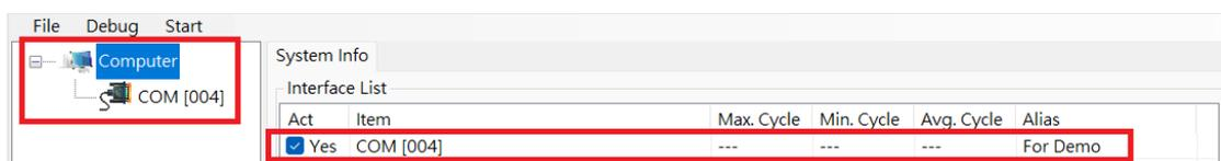
**Figure 4-10: The enable status of the new COM item in the Interface List**
