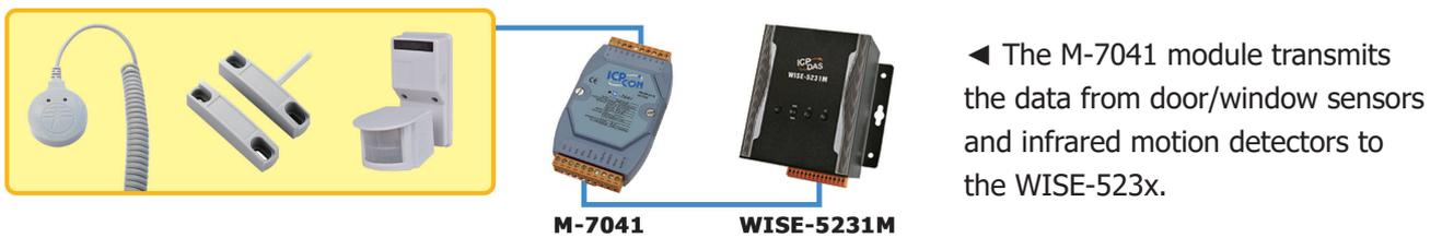
**WISE provides logic control to achieve the access control, camera capture and the alert notify of the mobile phone**
