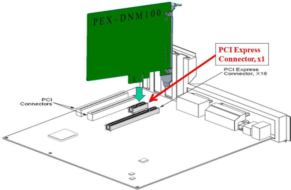
Figure 2.6 PEX-DNM100 installation
