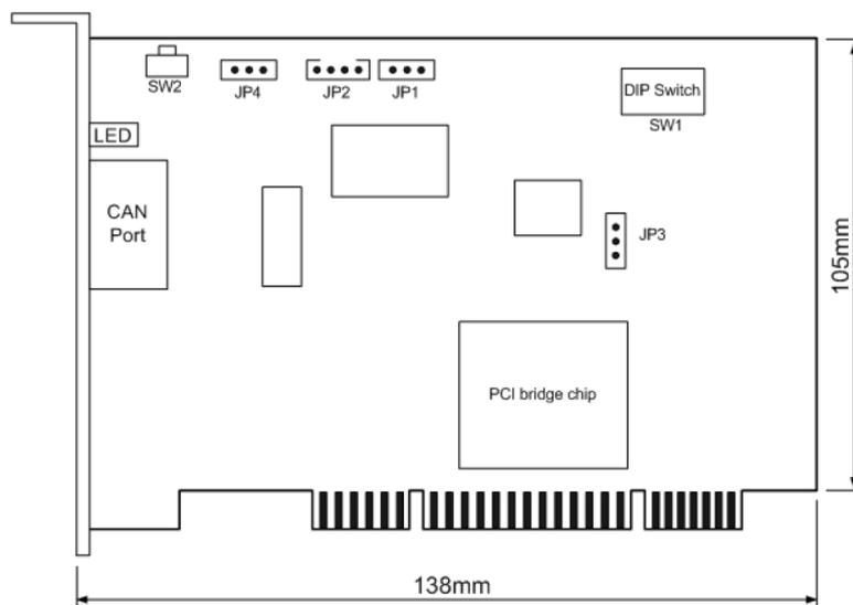
Figure 2.2 PISO-DNM100U Board Layout
