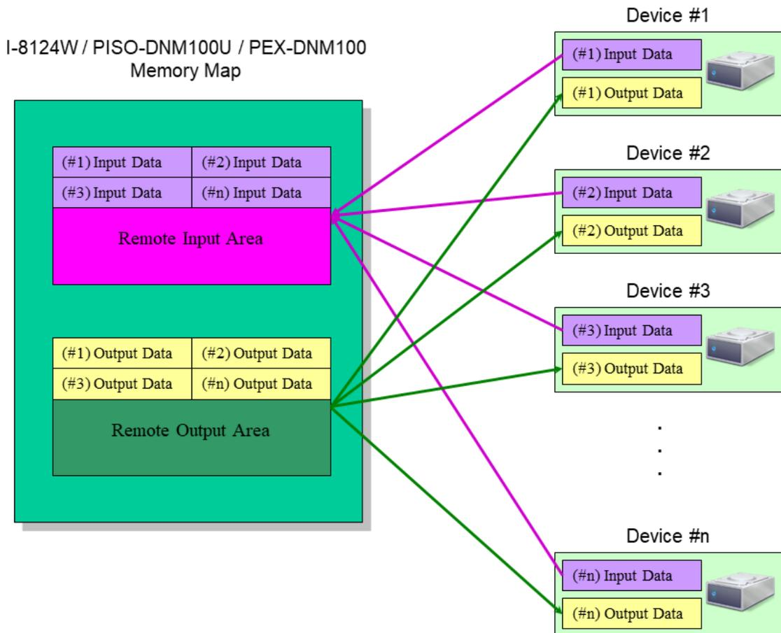
Figure 3.10 The Memory Mapping of the PISO-DNM100U or PEX-DNM100
