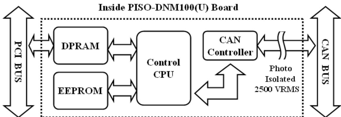
Figure 1.8 Block diagram of the PISO-DNM100U and PEX-DNM100
