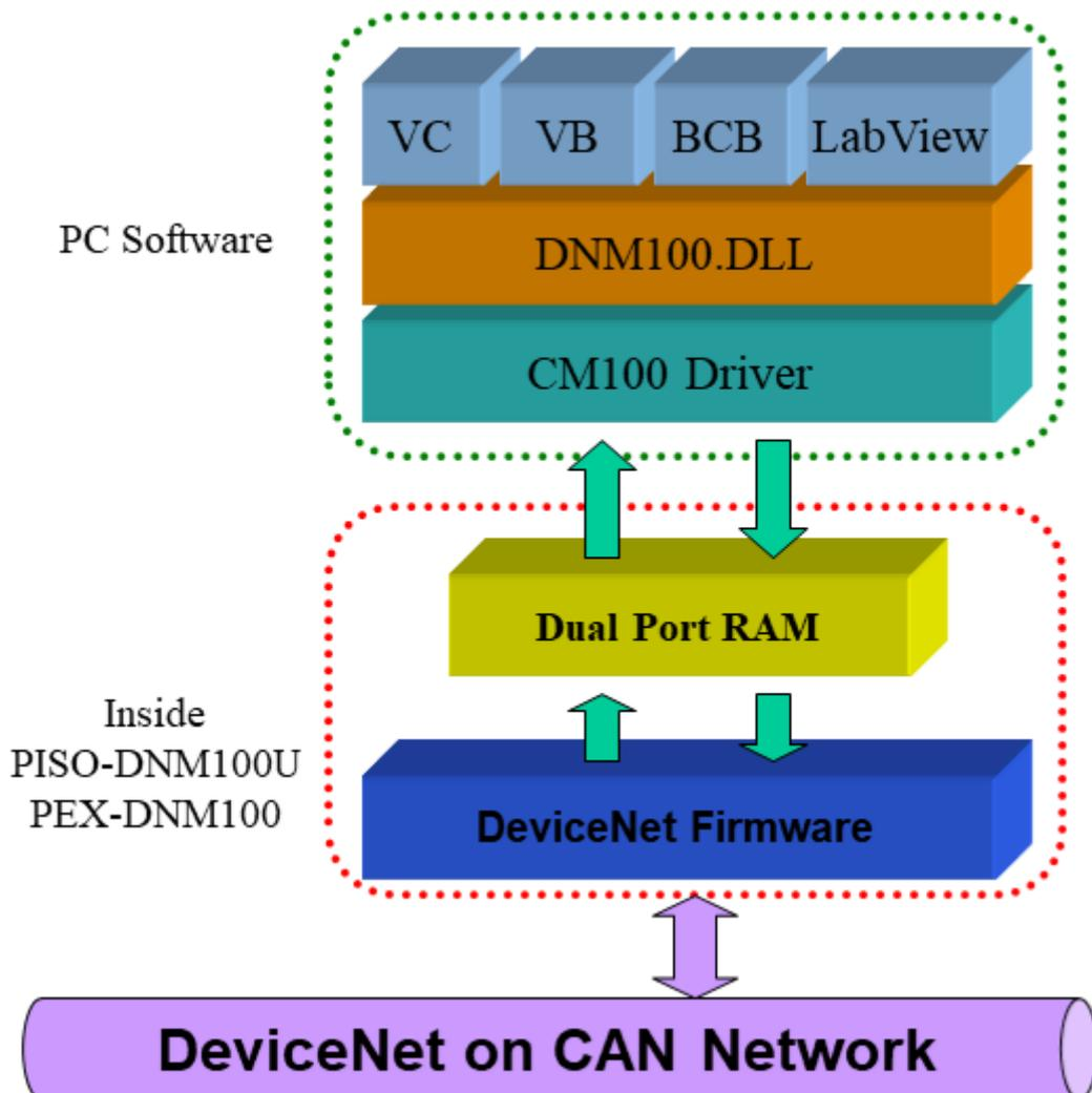
Figure 1.2 PISO-DNM100U and PEX-DNM100 illustration.
