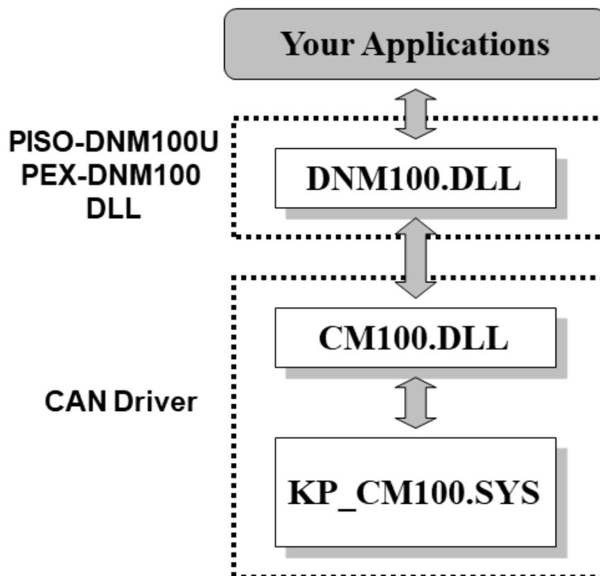
Figure 3.1 Software architecture in the Windows system
