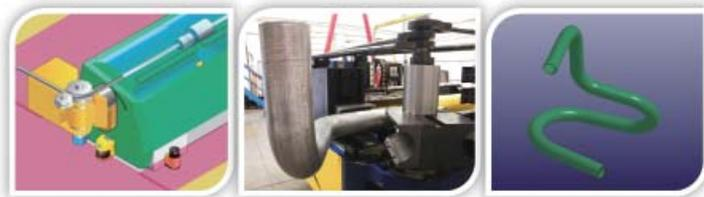
The CANopen motion library has included the CiA 402 profile. The users need not to care about the CANopen protocol and just focus on the control algorithm. The bender machine equipped the IPC and CANopen master PCI board (PISO-CPM100U). With the PISO-CPM100U and CANopen motion library, you can do various motion control functions, such as position control, velocity control, torque control, and synchronous action without having the background knowledge of the complex and abstruse CANopen protocol.
