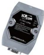
I-7565-CPM can represent an economic master solution of CANopen application. It follows CiA 301 specification such as, SDO, PDO, NMT, SYNC and so on. Besides, I-7565-CPM support EDS file interpretation, Heartbeat, Guarding, Slave Boot-up detection, and EMCY event functions. It is suited for portable diagnostic tool or main control unit of a CANopen network.
