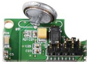
**Built-in RTC - Real Time Clock**
