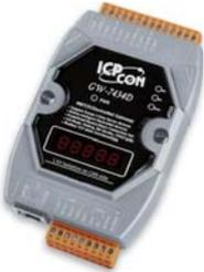
The GW-7434D is an economic solution that provides a communication protocol transformation between the DeviceNet protocol and the Modbus TCP protocol. This module solves the problem to connect an existing DeviceNet network to the Ethernet-based PLC, HMI or SCADA for setting up a control or monitoring system. The GW-7434D offers the Predefined Master connection Set function and Group 2 only Server function as a DeviceNet master.
