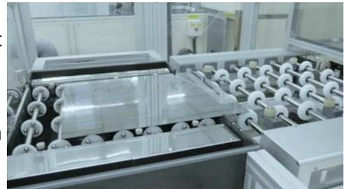
LCD glass plays an essential role in the entire production process of LCD panels, and the yield of glass substrates is even more important. The design of this system focuses on checking whether the glass has bubbles or cracks. The PISO-DNM100U controller is a perfect selection for use as a DeviceNet master device, utilizing only a small amount of CPU resources to achieve real-time control requirements, thereby improving product yield and system stability, together with excellent scalability.
