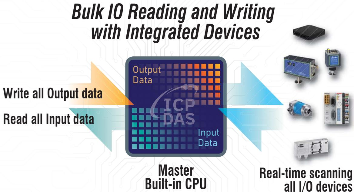
There are two memory areas in DeviceNet Master Series: one is "Remote Input Area" and the other is "Remote Output Area". The input data of all devices in the DeviceNet network will be placed in the "Remote Input Area"; the same, the output data will be concentrated in the "Remote Output Area". Users can read and write in these areas in one batch, which is equivalent to reading and writing to all remote devices.
