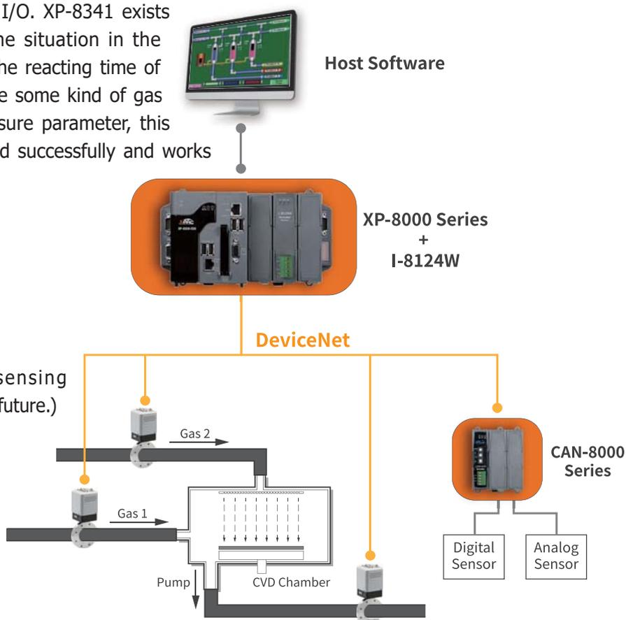
I-8124W is one of ICP DAS' DeviceNet Master product line, featuring high efficiency and high stability. It not only provides drivers for different platforms, but also provides DeviceNet development kits, which can freely develop monitoring software platforms and improve the application range of the overall system. This application in the monitoring system of the chemical vapor deposition machine not only improves the product yield and system stability, but also has system scalability.
