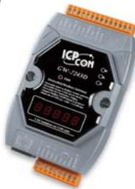
The GW-7243D offers the DeviceNet slave and Modbus master function. In the DeviceNet network, the module acts as a Group 2 Only Server device, and waits the connection with the DeviceNet master. In the Modbus network, the GW-7243D is a master device, and cyclically access the Modbus slave devices. Both the Modbus TCP client and Modbus RTU/ASCII master interfaces of the GW-7243D can work simultaneously. This is helpful to build the applications easily and quickly.
