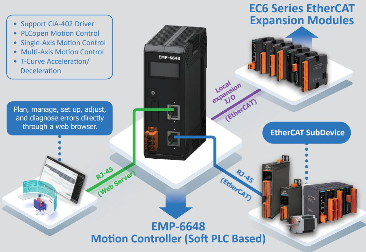
▲ The EMP-6648 offers multiple EtherCAT subdevice connection options. Users can expand via EC6 series modules or RJ-45 connectors to maximize space utilization, achieve high-density I/O configuration, maintain a compact size, and enable flexible scalability.
