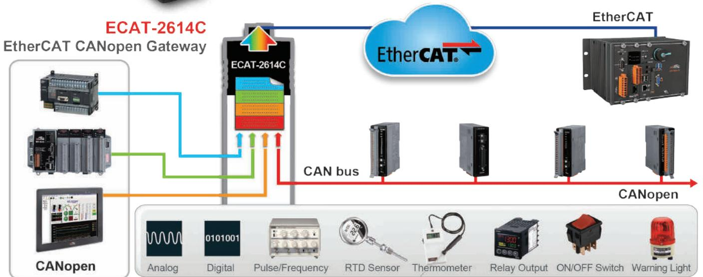
▲ Anything can be connected to the EtherCAT Main Device via ECAT-2614C as long as it is a CANopen device
