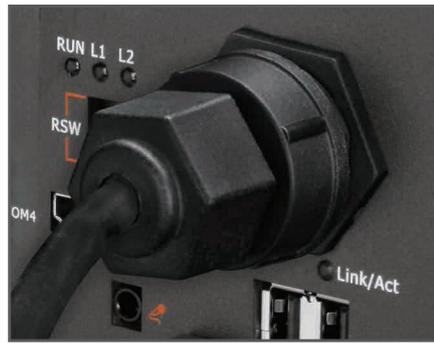
▲ Secured RJ45 Connector Kit
