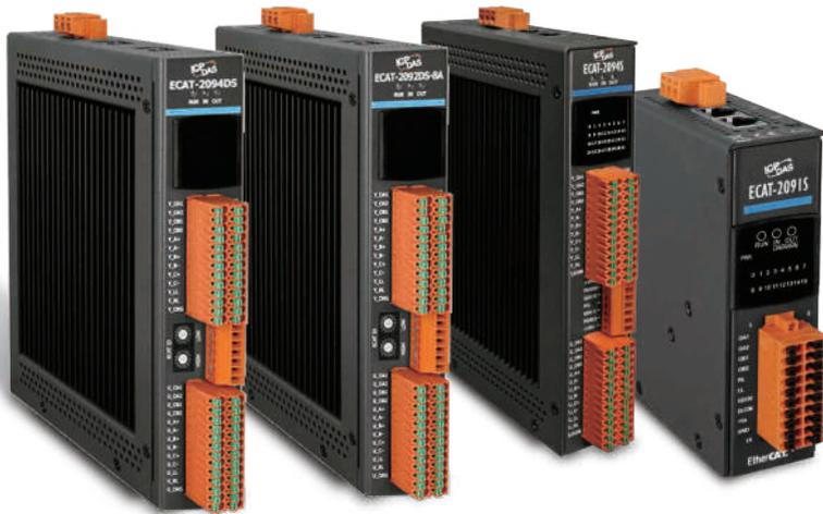
ICP DAS stepping motor controllers are designed for two-phase bipolar motors using open-loop control. They support up to four-axis synchronized control, the CiA402 protocol, and programmable current control up to 8A. They also offer a range of protective, stabilized, and precise control functions.
