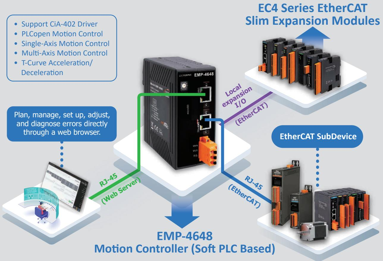
▲ The EMP-4648 offers multiple EtherCAT subdevice connection options. Users can expand via EC4 series modules or RJ-45 connectors to maximize space utilization, achieve high-density I/O configuration, maintain a compact size, and enable flexible scalability.
