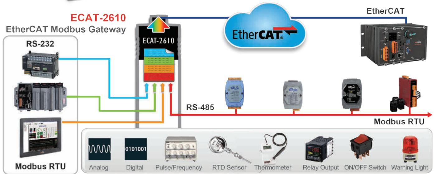
▲ Anything can be connected to the EtherCAT Main Device via ECAT-2610 as long as it is a Modbus RTU device
