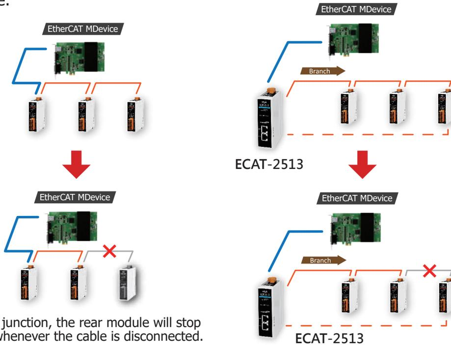
▲ Without a junction, the rear module will stop working whenever the cable is disconnected.
