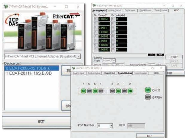
▲ iECAT Utility ICP DAS EtherCAT Module Verification and Adjustment Tool
