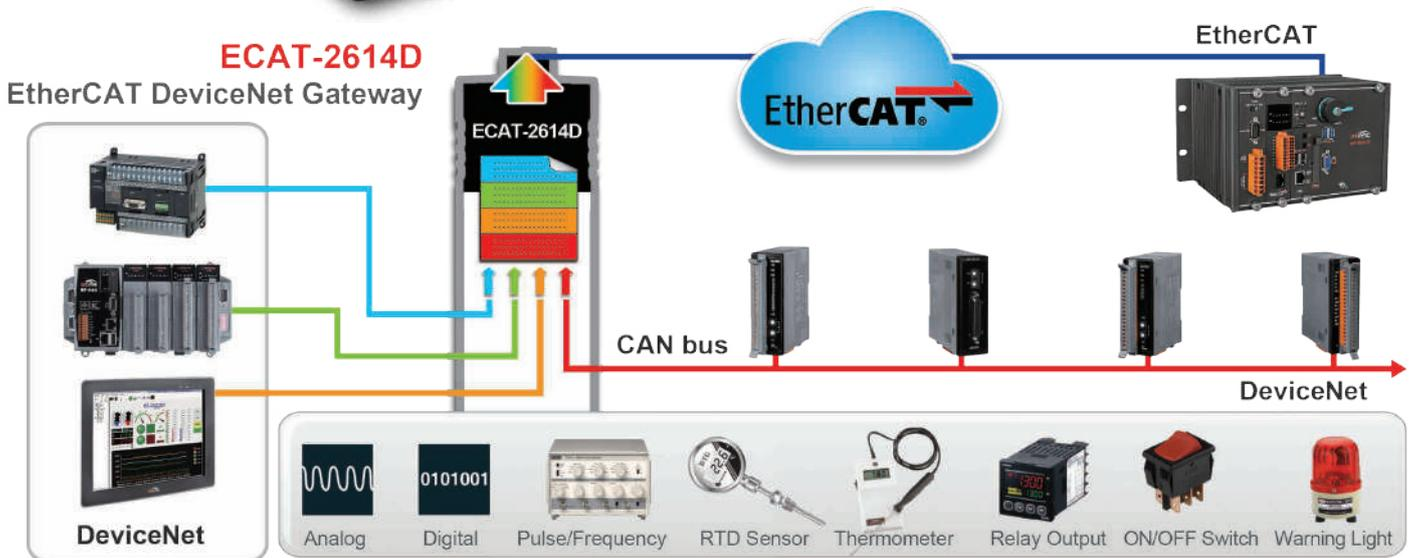
▲ Anything can be connected to the EtherCAT Main Device via ECAT-2614D as long as it is a DeviceNet device
