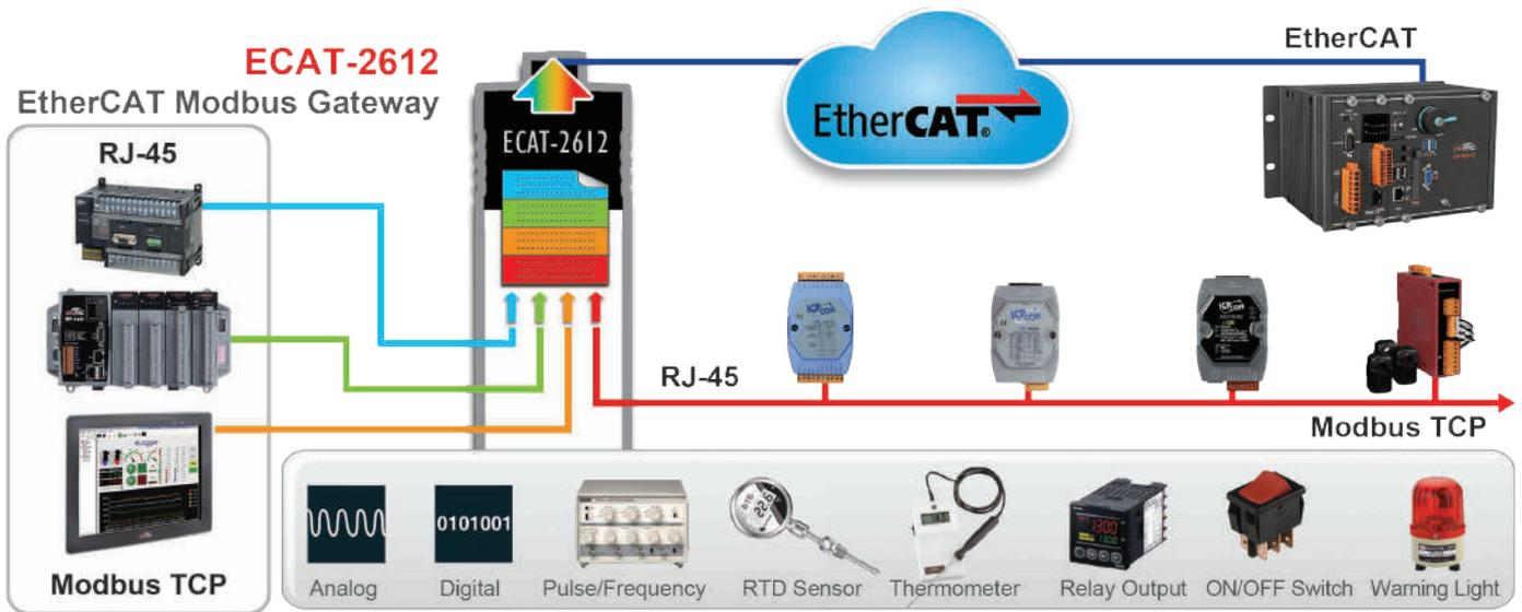
▲ Anything can be connected to the EtherCAT Main Device via ECAT-2612 as long as it is a Modbus TCP device
