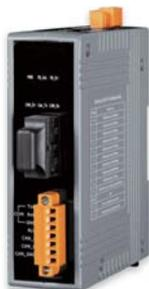
The I-2533CS-FD is a local CAN FD bridge used to establish a connection between two CAN FD system via single mode fiber optic transmission medium. In order to solve the problem between CAN FD and fiber transmission medium, the I-2533CS-FD is specially designed for converting the electrical CAN FD signal to fiber optic cables.
