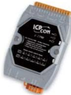
The GW-7828 gateway is a Modbus RTU slave device that allows the Modbus RTU master to access the M-Bus slave devices. These M-Bus devices may be a water meter, electric meter, power meter and so forth. Owing to the GW-7828, you can put the M-Bus slave devices into Modbus network very easily.
