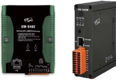
GW-5492, GW-5493, GW-2492M and GW-2493M is a fully configurable universal BACnet/IP to Modbus RTU/TCP gateway. The GW-549x and GW-249xM include BACnet/IP Server and Modbus RTU Master (GW-5492/2492M) or TCP Client (GW-5493/2493M) which is used to make Modbus devices accessible on a BACnet network.
