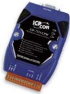
The GW-7553-CPM is designed for the slave device of PROFIBUS DP protocol. It allows PROFIBUS master to access CANopen slave devices. These CANopen slave device may be a sensor, actuators, ICPDAS CAN-2000 series modules and so forth. In addition, we also provide the utility software for users to configure the GW-7553-CPM. By using this module, users can put their CANopen slave devices into PROFIBUS network very easily.
