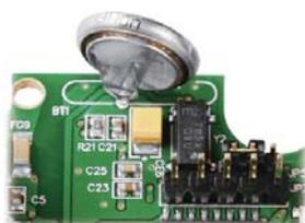
Built-in RTC - Real Time Clock
