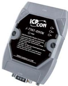
I-7565-DNM can represent an economic master solution of DeviceNet application. It is a "Predefined Master-Slave connection Set". I-7565-DNM supports Group 2 only Server and UCMM functions to communication with slave devices. It has an independent CAN Bus communication port to cover a wide range of DeviceNet applications.
