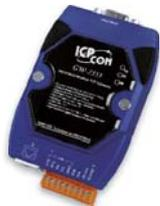
The GW-7553 is used for data-exchange between the Modbus TCP/RTU network and the PROFIBUS network. It provides not only the Modbus TCP client and server functions, but the Modbus RTU master and slave functions. Therefore, the GW-7553 can satisfy most of the applications of the data transfer between Modbus and PROFIBUS.
