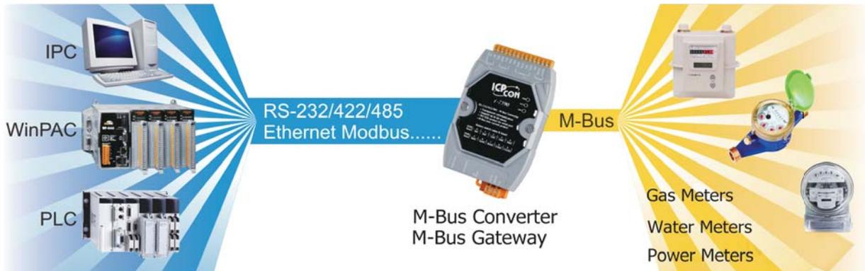
The M-Bus ("Meter-Bus") is a European standard for remote reading of meters. It is usable for most types of consumption meters as well as for various sensors and actuators.
