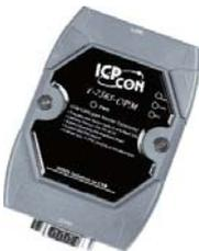
I-7565-CPM can represent an economic master solution of CANopen application. It follows CiA 301 specification such as, SDO, PDO, NMT, SYNC and so on. Besides, I-7565-CPM support EDS file interpretation, Heartbeat, Guarding, Slave Boot-up detection, and EMCY event functions. It is suited for portable diagnostic tool or main control unit of a CANopen network.
