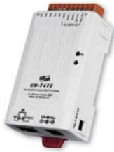
The GW-7472 (EtherNet/IP adapter to Modbus TCP/RTU Master Gateway) is helpful for data-exchanging between the Modbus RTU Network, Modbus TCP Network, and the EtherNet/IP Network. It reads the register data from the Modbus RTU slaves as well as Modbus TCP servers and publishes these data to the input register data of the EtherNet/IP scanner. The output data transmitted by the EtherNet/IP scanner are updated to the register data of Modbus TCP/RTU slaves via the GW-7472.
