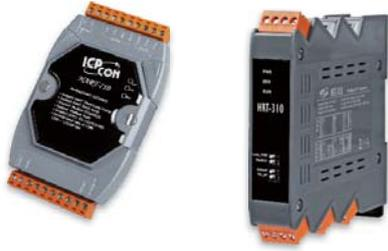
The HRT-710/HRT-310 is a Modbus RTU/ASCII slave to HART master gateway. It provides an economic solution for Modbus master device to access the HART slave devices. In order to diagnose and configure the HART network more easily, the HG\_Tool Utility with friendly configuration interface is given.
