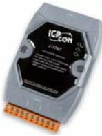
I-7567 is a USB to HART converter specially designed as the master device of HART protocol. Through it, users can easily access the HART network via USB port which is implemented as a virtual COM port on PCs or notebooks. Because the I-7567 is powered by the USB interface, the external power is not necessary. Moreover, the I-7567 provides the Utility tool which is helpful for diagnosing and configuring the HART network.
