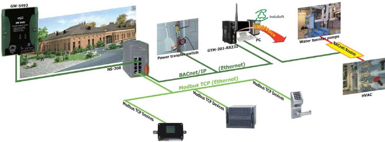
Airconditioning Data Acquisition System
