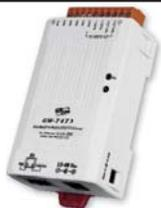
The GW-7473 (Modbus TCP/RTU Slave to EtherNet/IP Scanner Gateway) is helpful for data-exchanging between Modbus Master and EtherNet/IP adapter. It reads the register data from the EtherNet/IP adapter and publishes these data to the input register data of the Modbus TCP client as well as Modbus RTU Master. The output data transmitted by the Modbus TCP/RTU Master are updated to the register data of EtherNet/IP adapter.
