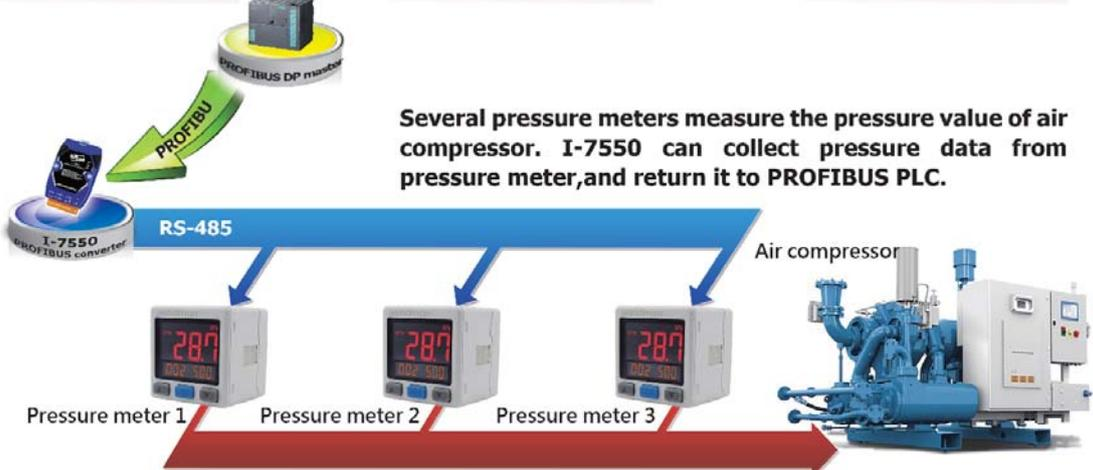
Several pressure meters measure the pressure value of air compressor. I-7550 can collect pressure data from pressure meter, and return it to PROFIBUS PLC.
