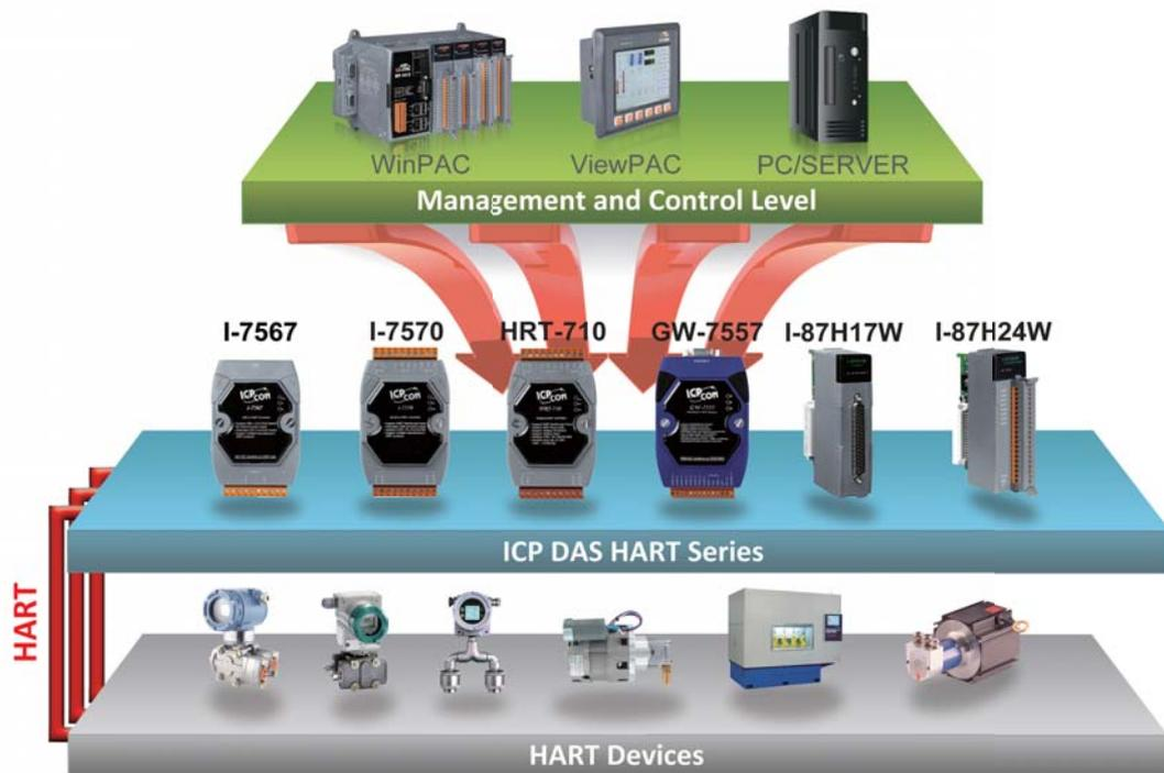
The following diagram will illustrate the HART bus applications and understand the roles of ICP DAS HART communication modules in HART network.
