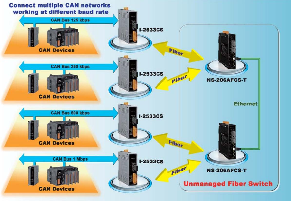
**I-2533CS-A I-2533CS-B CAN to Multi-mode Fiber Bridge**
