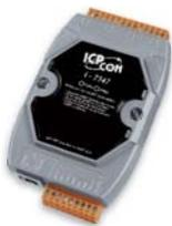
The I-7547 is an Ethernet to HART converter designed as the master device of HART protocol. It allows users to access the HART slave via Ethernet. These HART slave devices may be a transmitter, actuator, current output device and so forth. In addition, by using the HC\_Tool utility, users can configure module and test HART communication easily and quickly.
